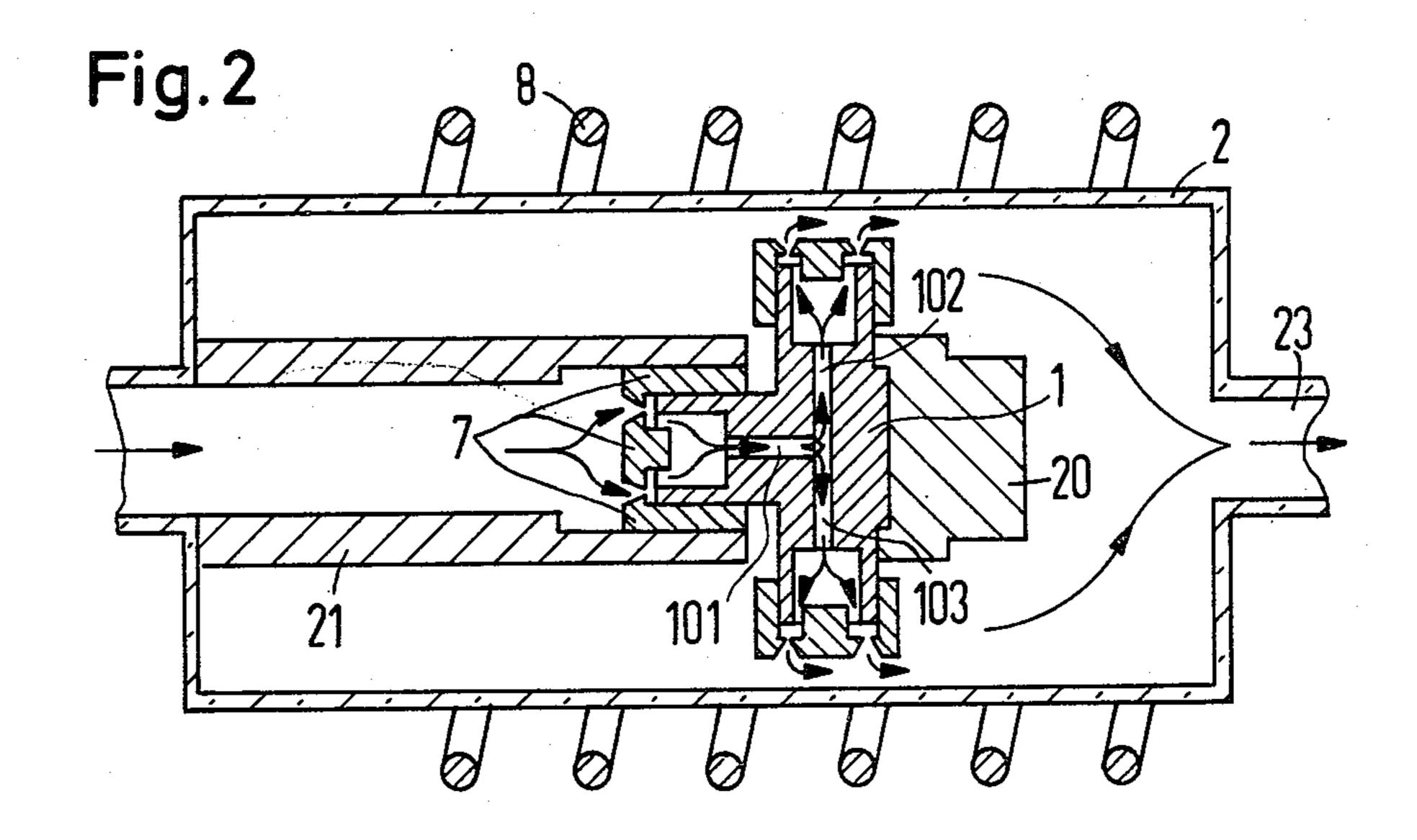
METHOD FOR DEPOSITING A LAYER ON THE INSIDE OF CAVITIES OF A WORK PIECE
