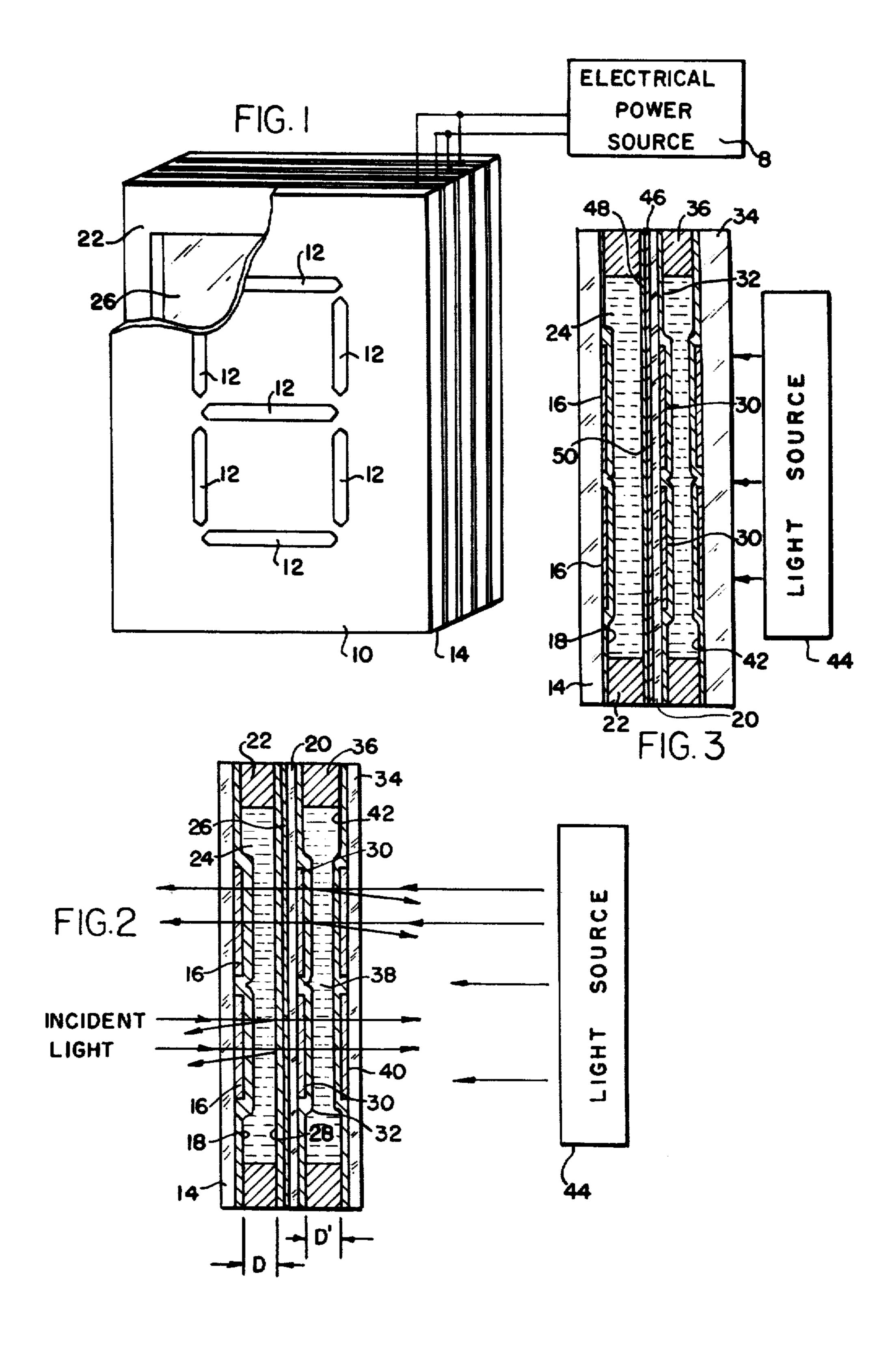
incident light producing a visible image at the front face of the display panel.
