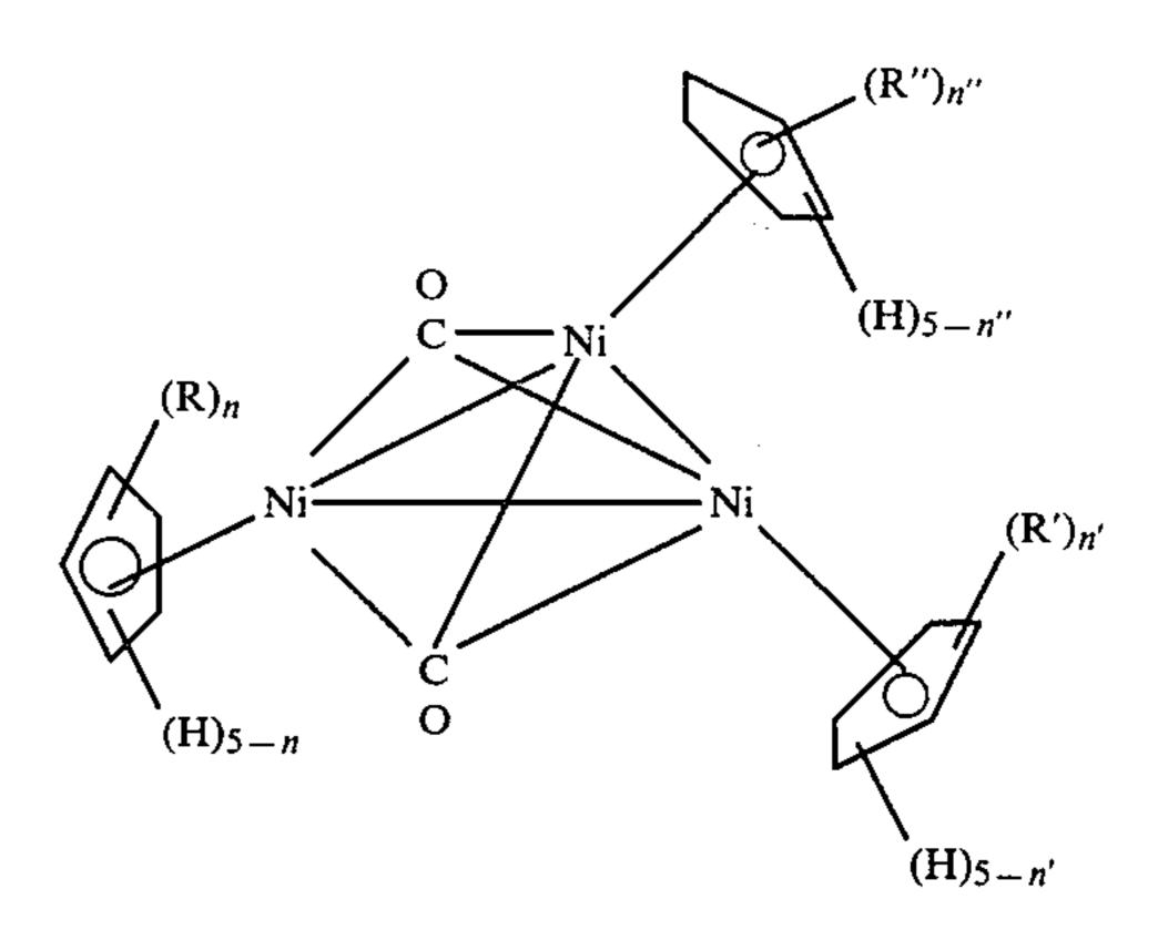
wherein R, R' and R" are the same or different C<sub>1</sub> to C<sub>20</sub> hydrocarbon radicals and n, n' and n" can be the same or different integers of 0 to 5, inclusive.
