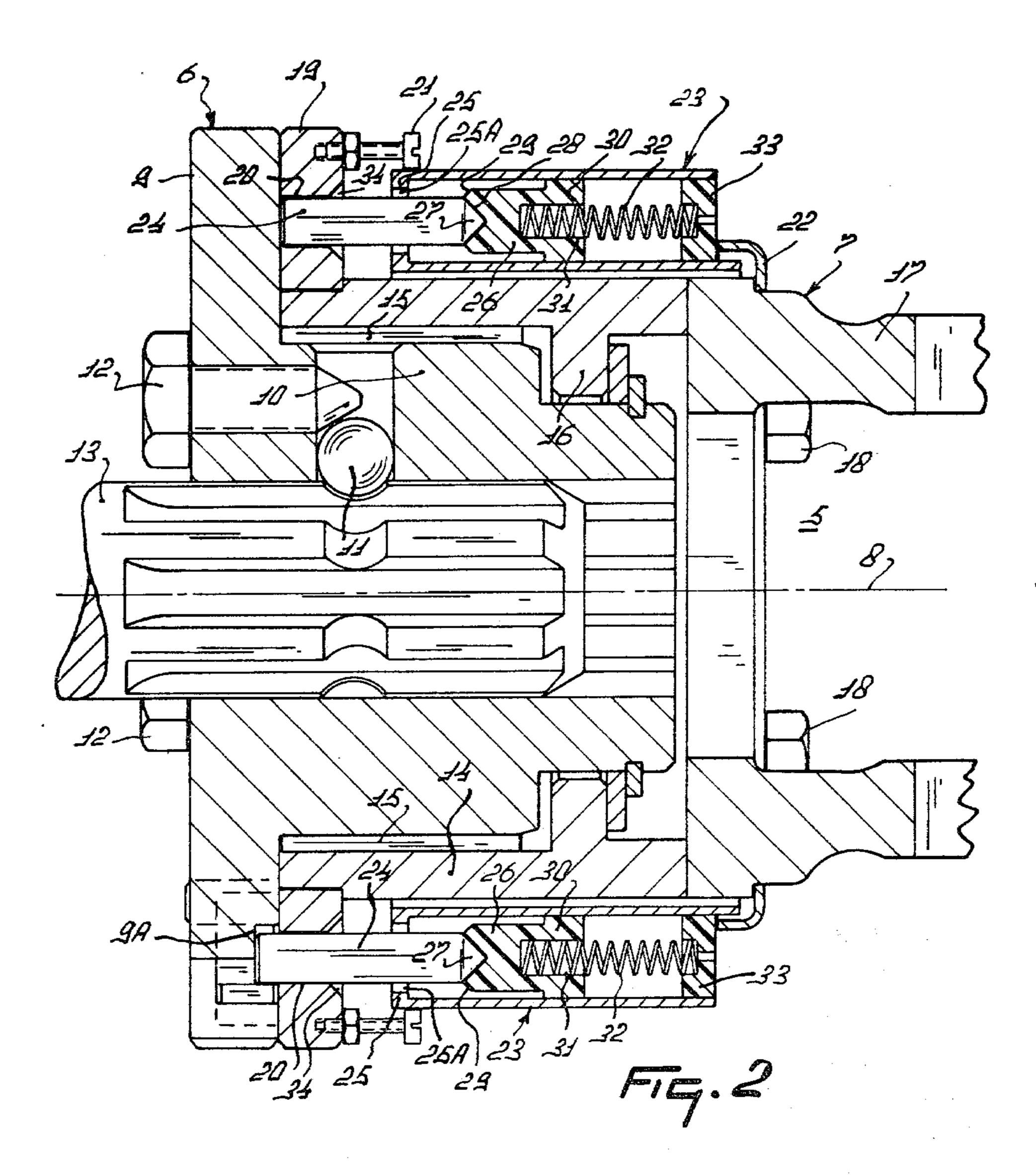
invention relates to a shear pin coupling
