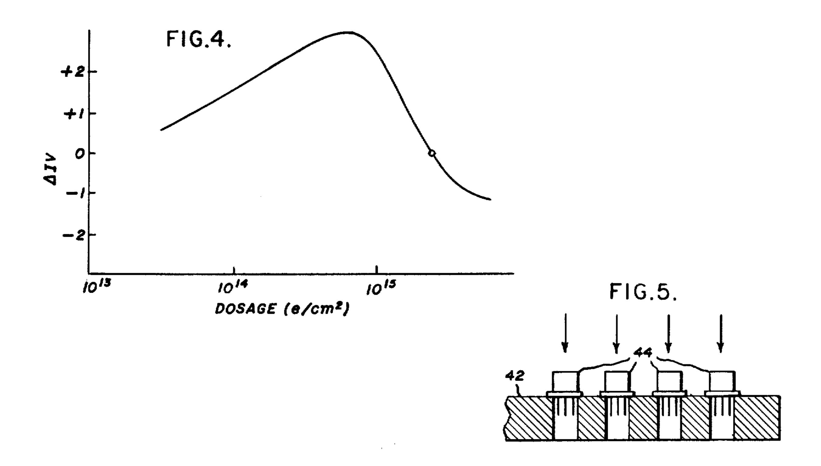
CONTROL OF VALLEY CURRENT IN A UNIJUNCTION TRANSISTOR BY ELECTRON IRRADIATION
