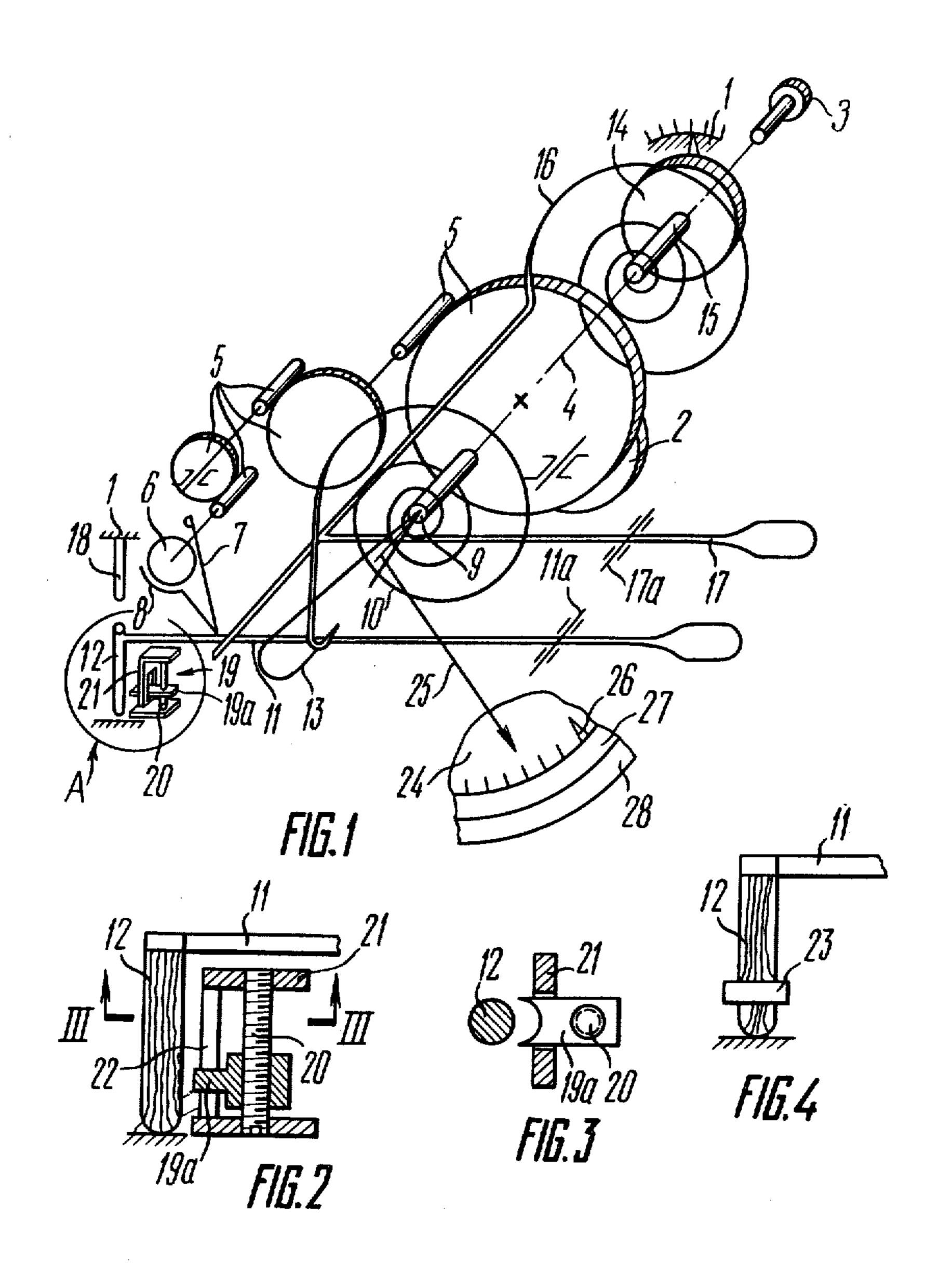
APPARATUS WITH A PERMANENT MAGNET FOR GAUGING THE THICKNESS OF COATINGS ON METAL PRODUCTS WITH MAGNETIC SHUNT TO ADJUST FOR DEMAGNETIZATION OF THE PERMANENT MAGNET
