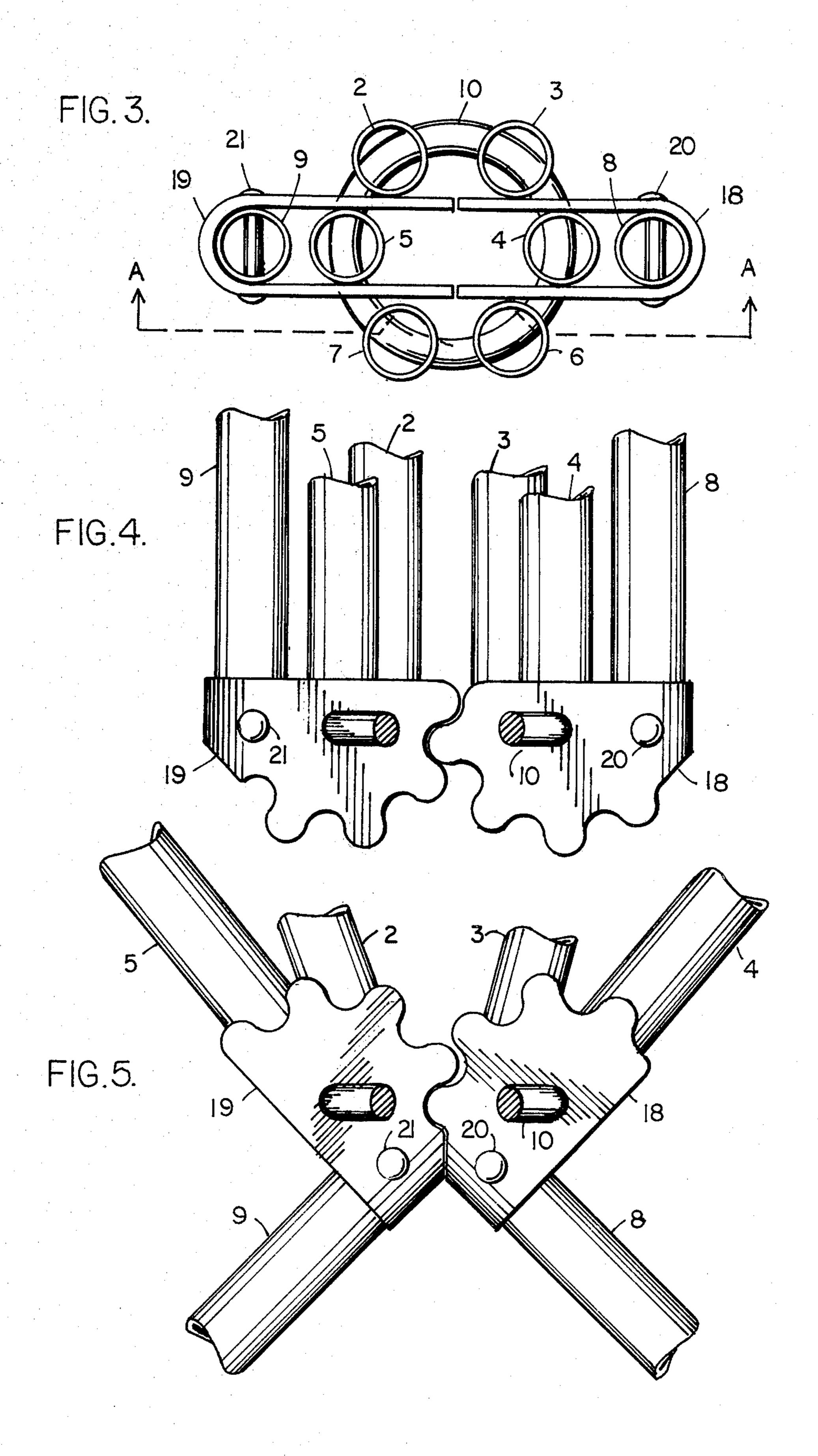
This invention relates to seating structures and is particularly concerned with lightweight and compactly 5 folding chairs wherein the support elements, when the chair is folded, are brought together into a close parallel relationship, the seat back, arms, and base being composed of a fabric or similar flexible material.
