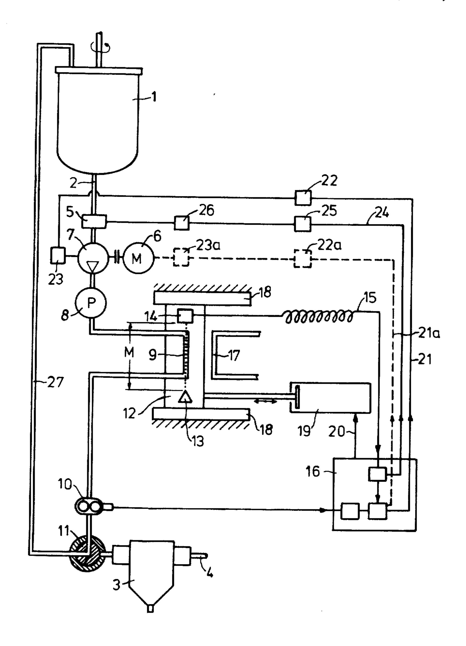
METHOD AND A DEVICE FOR THE PRODUCTION OF A SOLID-FORMING OR FOAM-FORMING FLOWABLE REACTION MIXTURE
