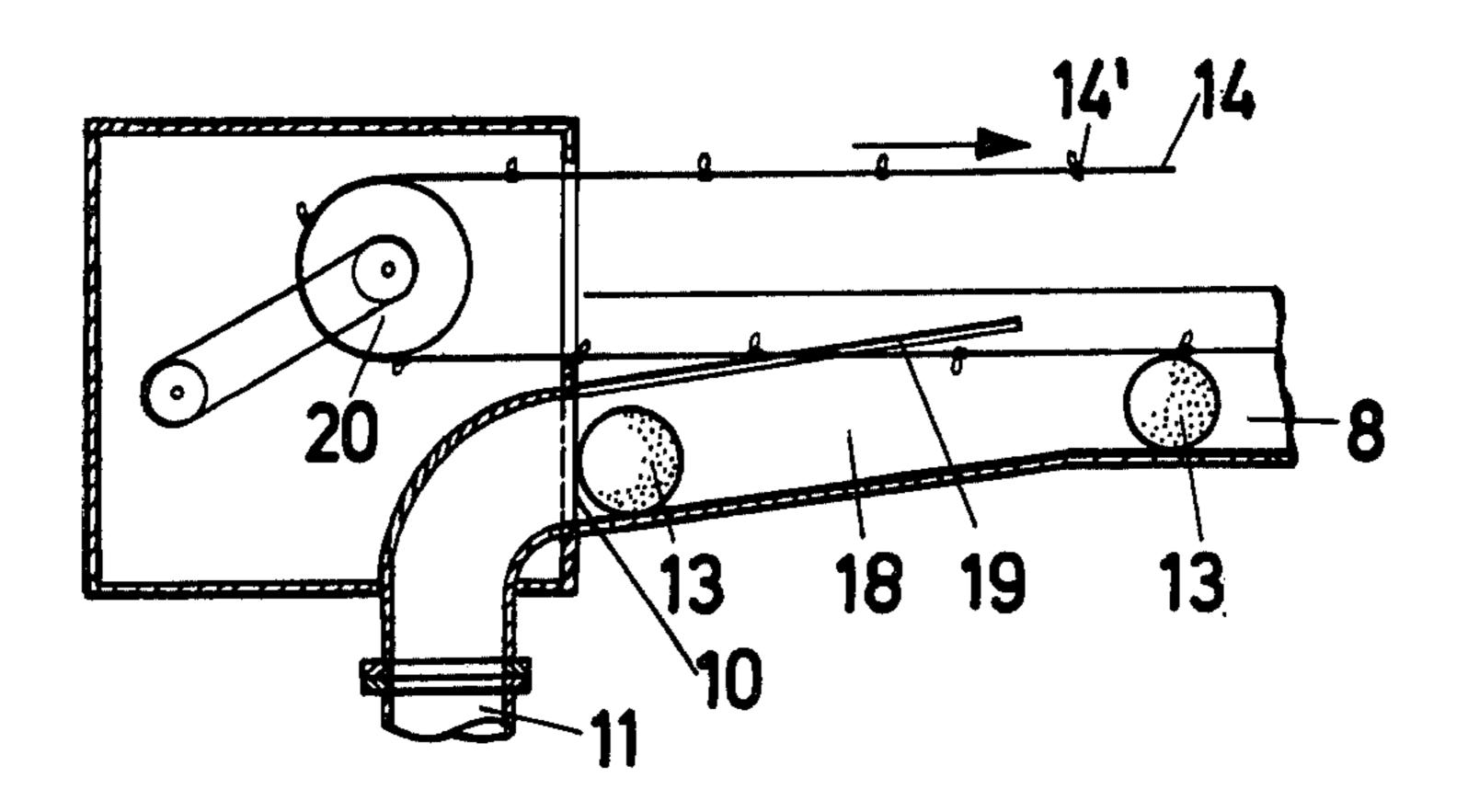
(b) the collecting chute has a downwardly sloping section only at one end adjacent to the withdrawal point and is provided above the downwardly sloping section with at least two guide members adapted to deflect the balls downwards, the run of the conveyor
