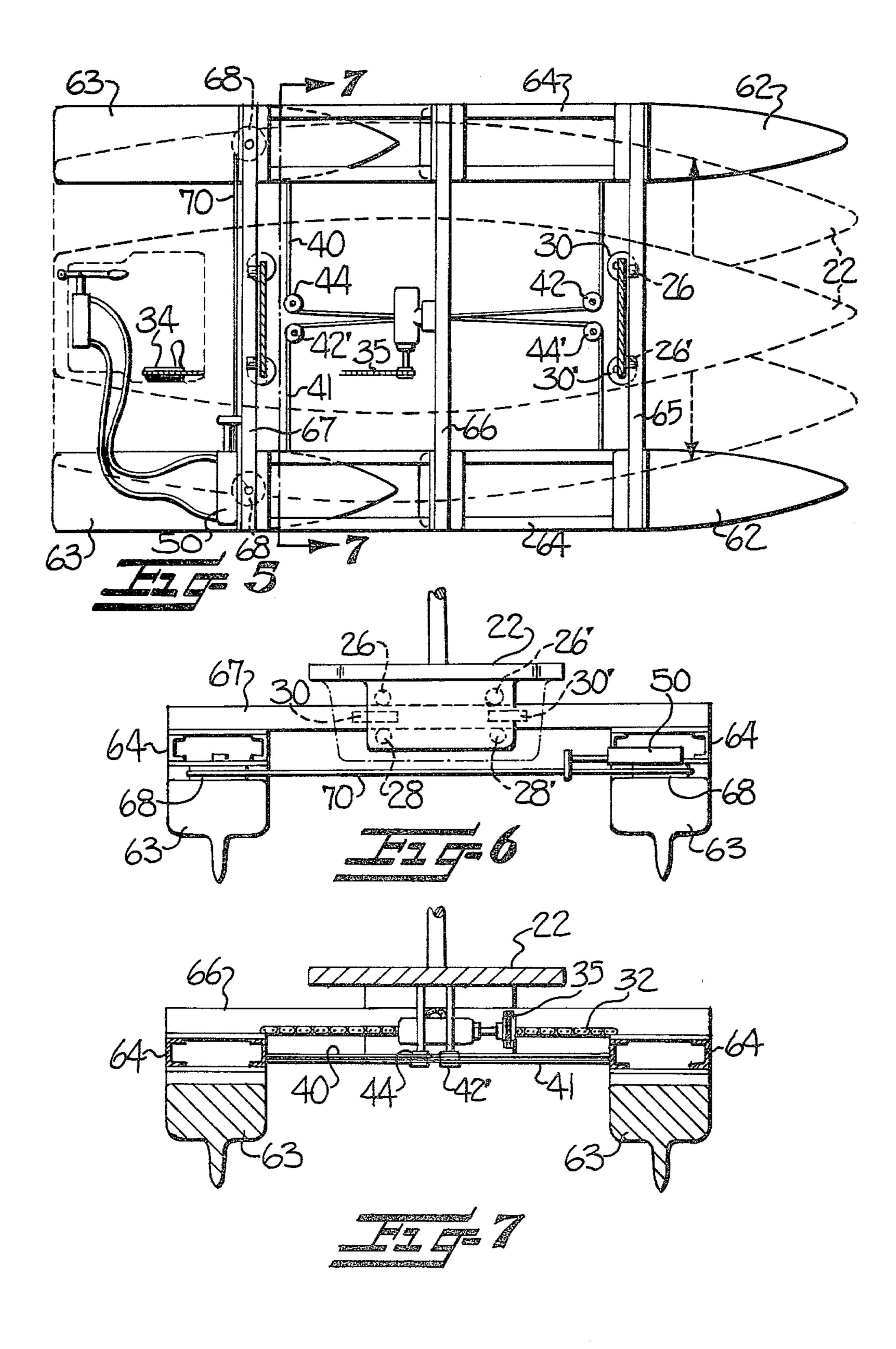
of the hulls comprises a pair of longitudinally spaced apart hull sections, and the rearward hull section of
