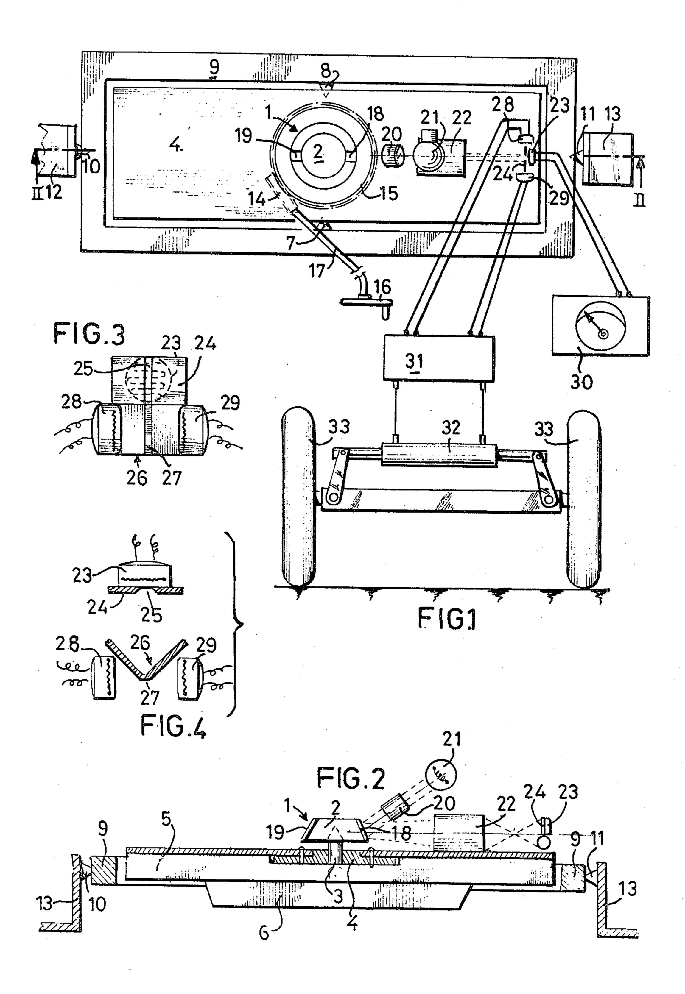
DEVICE FOR GUIDING THE DISPLACEMENT OF A VEHICLE AND IN PARTICULAR AN AGRICULTURAL MACHINE
