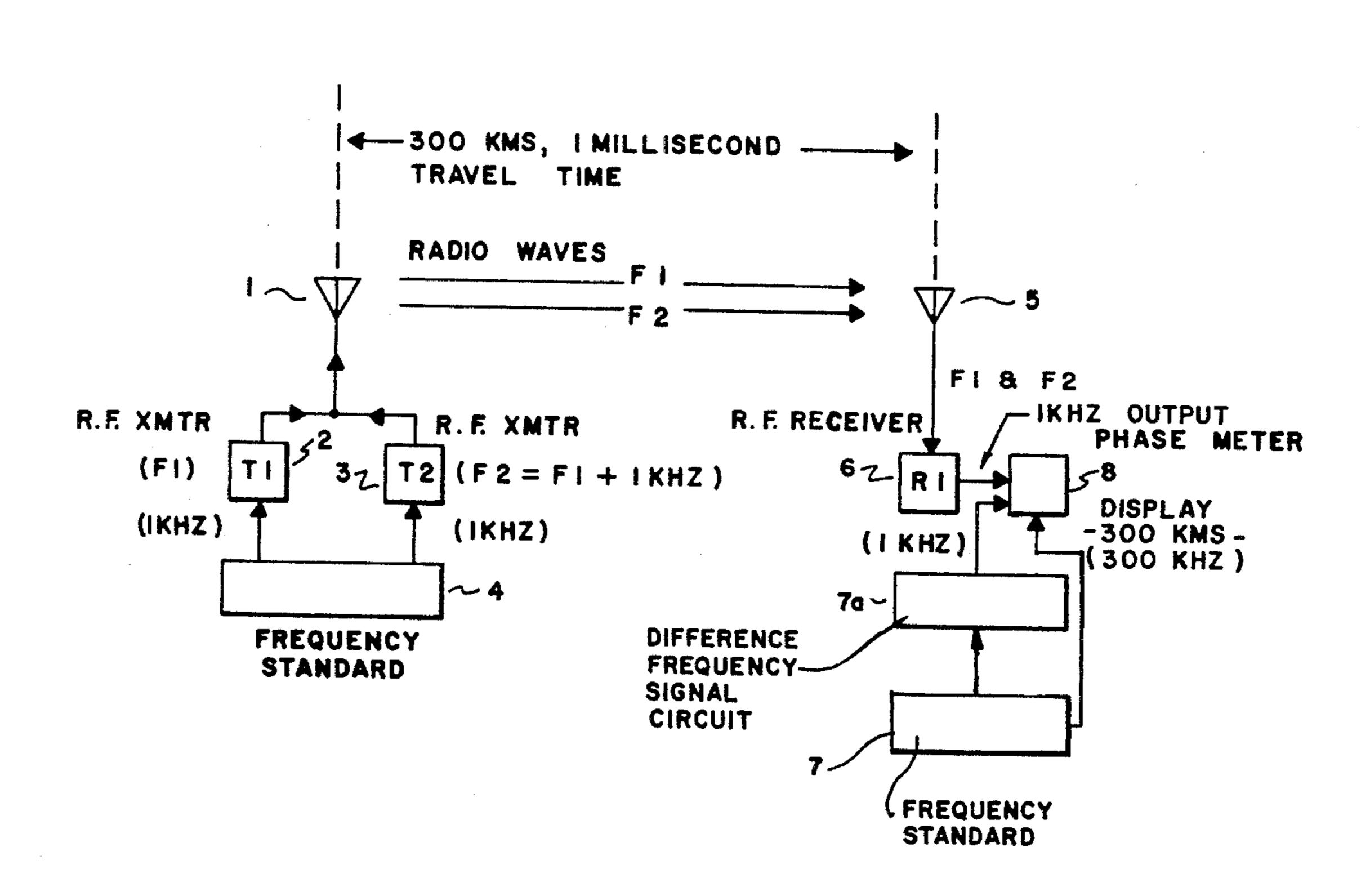
FIGURE NO. I MEASURING DISTANCE BY RADIO MEANS (2 FREQUENCY METHOD )
