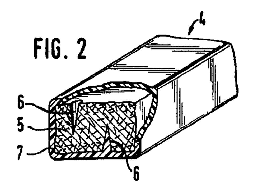
COMPOSITE MATERIAL WITH A CORE AND AN ADHERING COATING UNITED THERETO
