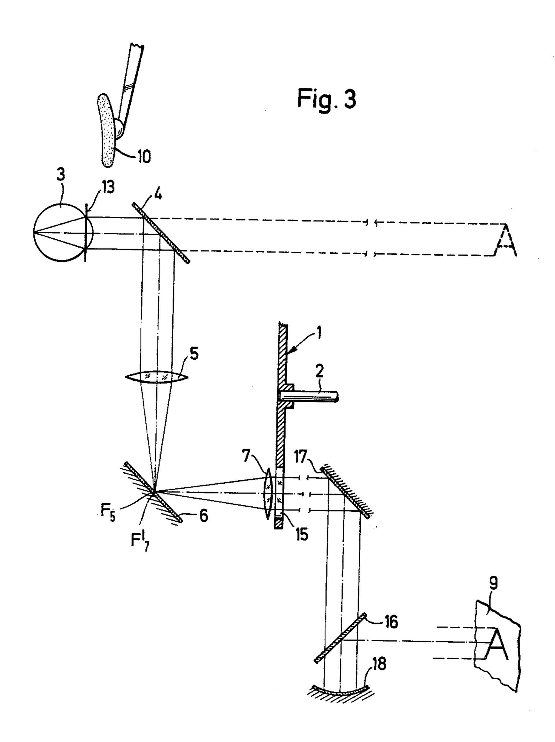
The principal rays 11 in the beam path are illustrated by means of the thick solid lines and the secondary rays 12 are illustrated by means of the thin solid lines.
