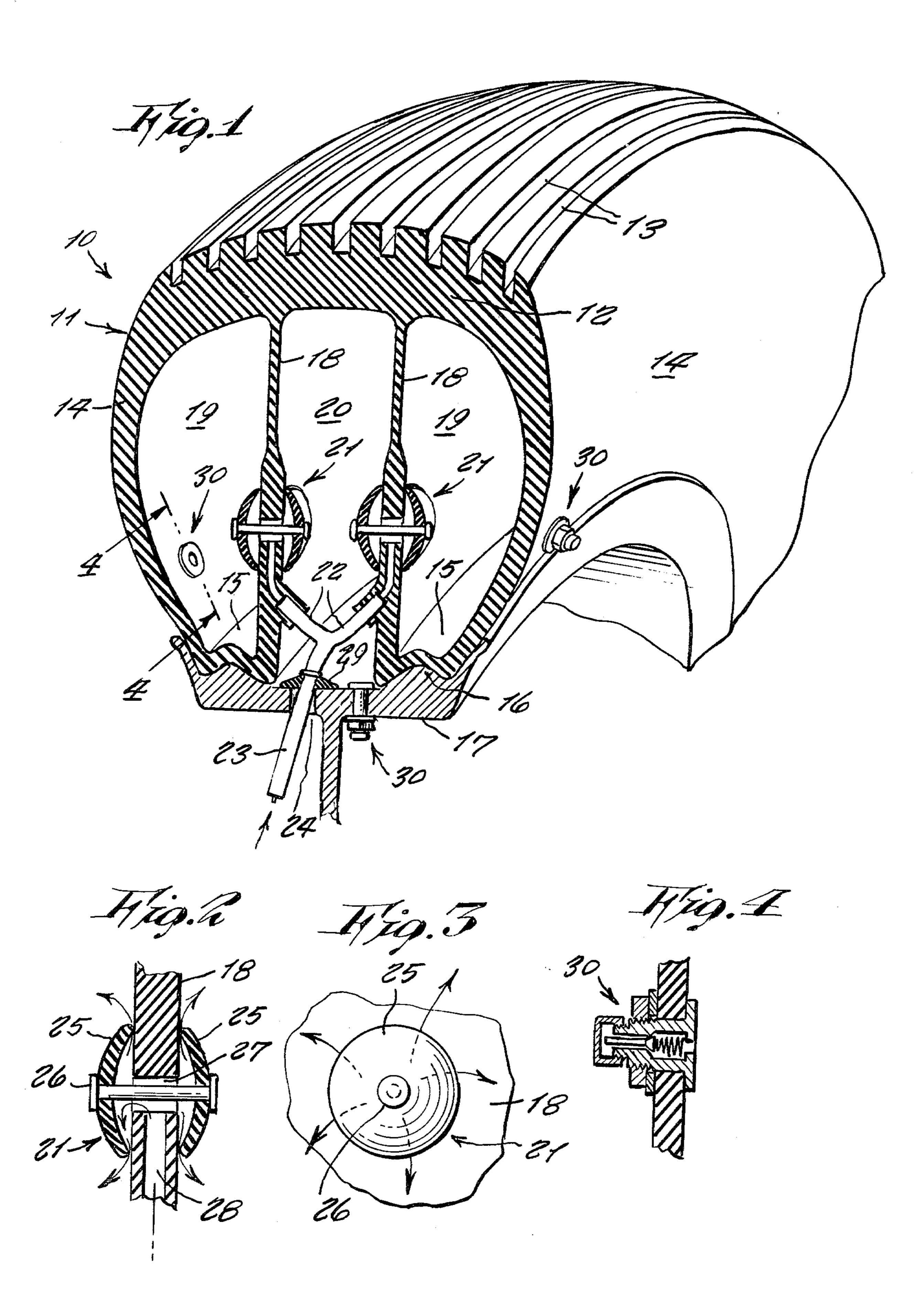
integral with the inner wall 15. Thus the side chambers 19 are each sealed due to the inner wall 15, while a central chamber 20 is open at its radially inward end, but which becomes sealed by the wheel when the tire is mounted thereupon.
