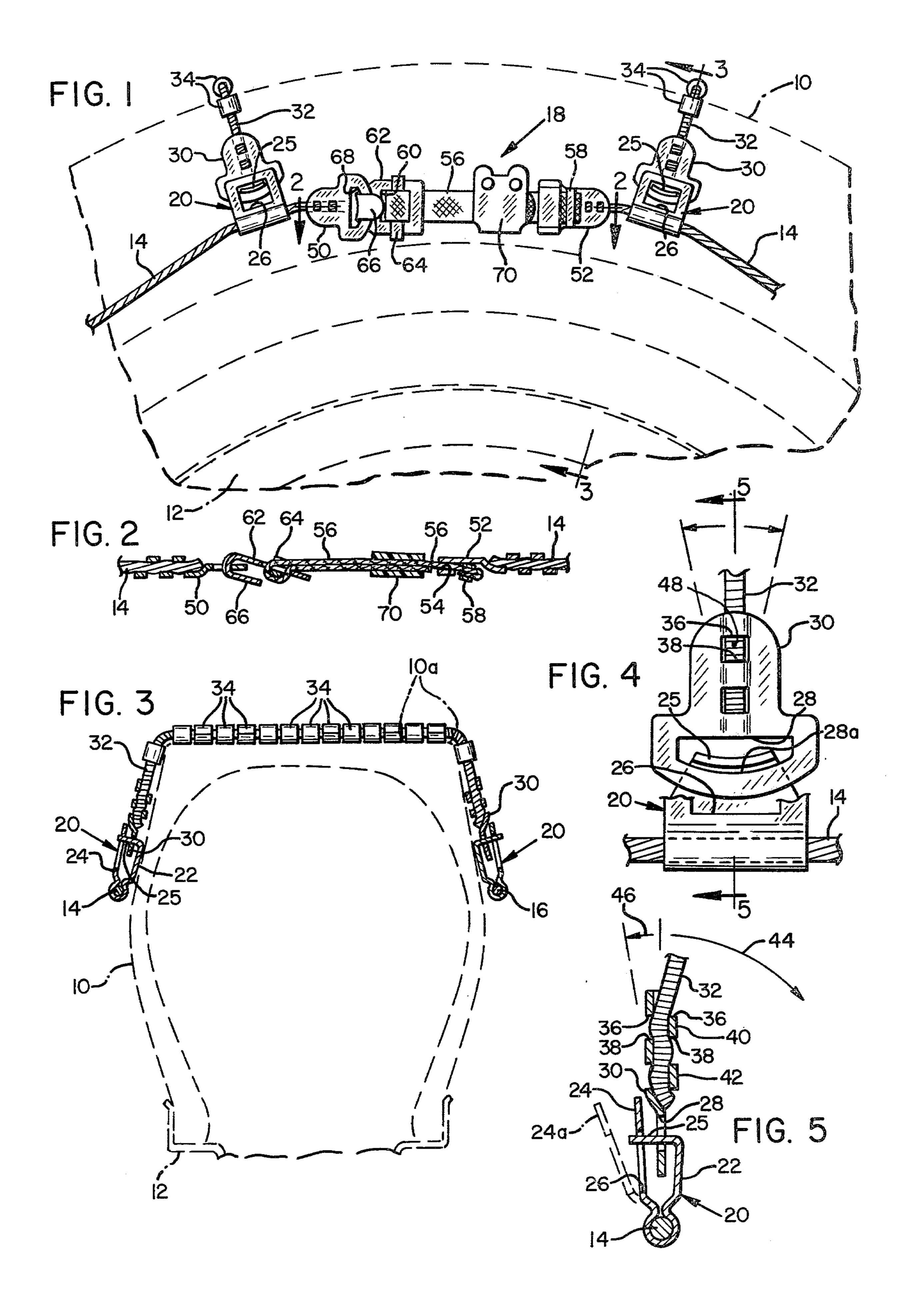
WIRE ROPE TRACTION DEVICE FOR TIRES
