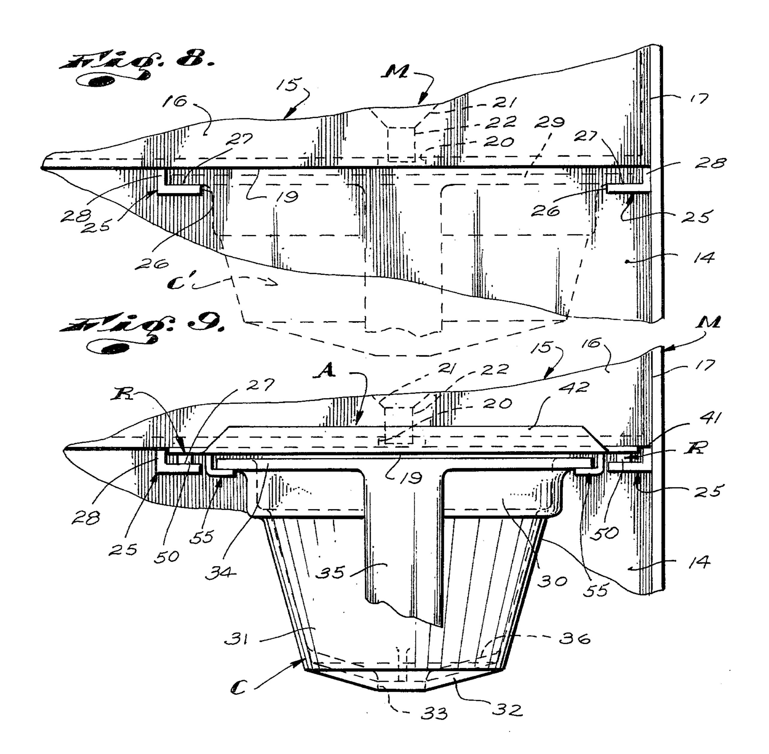
through the bed of ground coffee beans within the cone, extracting flavor and essence therefrom. The coffee brewed within the cone flows out through the opening in the bottom thereof and into the decanter.
