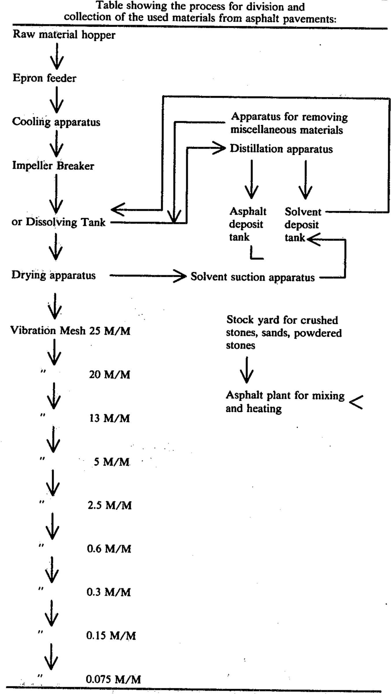
rated by distillation may be collected almost in a state of pure asphalt and is deposited in an asphalt deposit or 65 storage tank. The solvent is separately deposited in a solvent deposit tank. In this case, the solvent thus separately deposited may be returned to the dissolving tank
