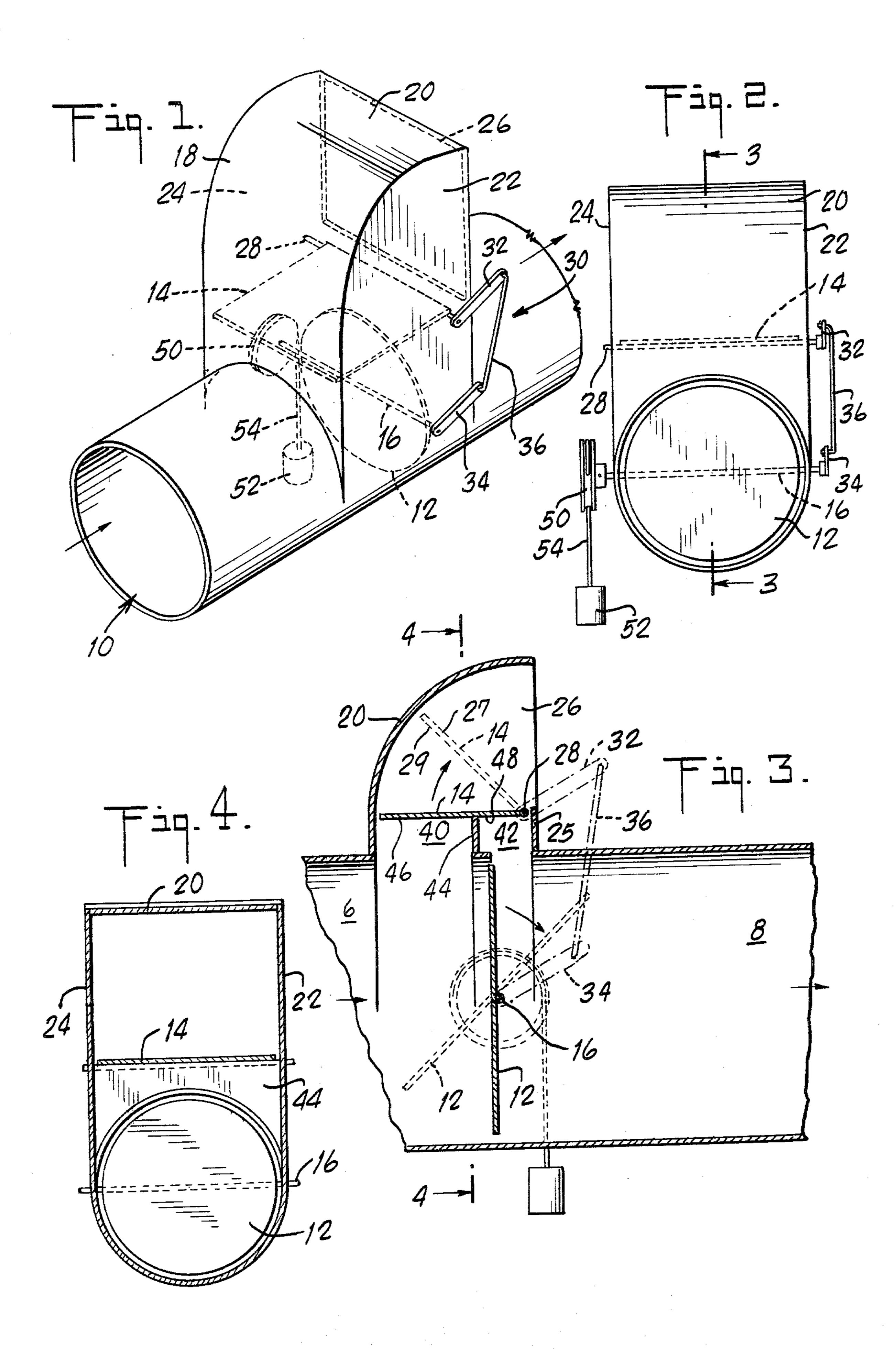
tion provides a positive closing action for the damper without assistance from an external power source when the burner shuts off.
