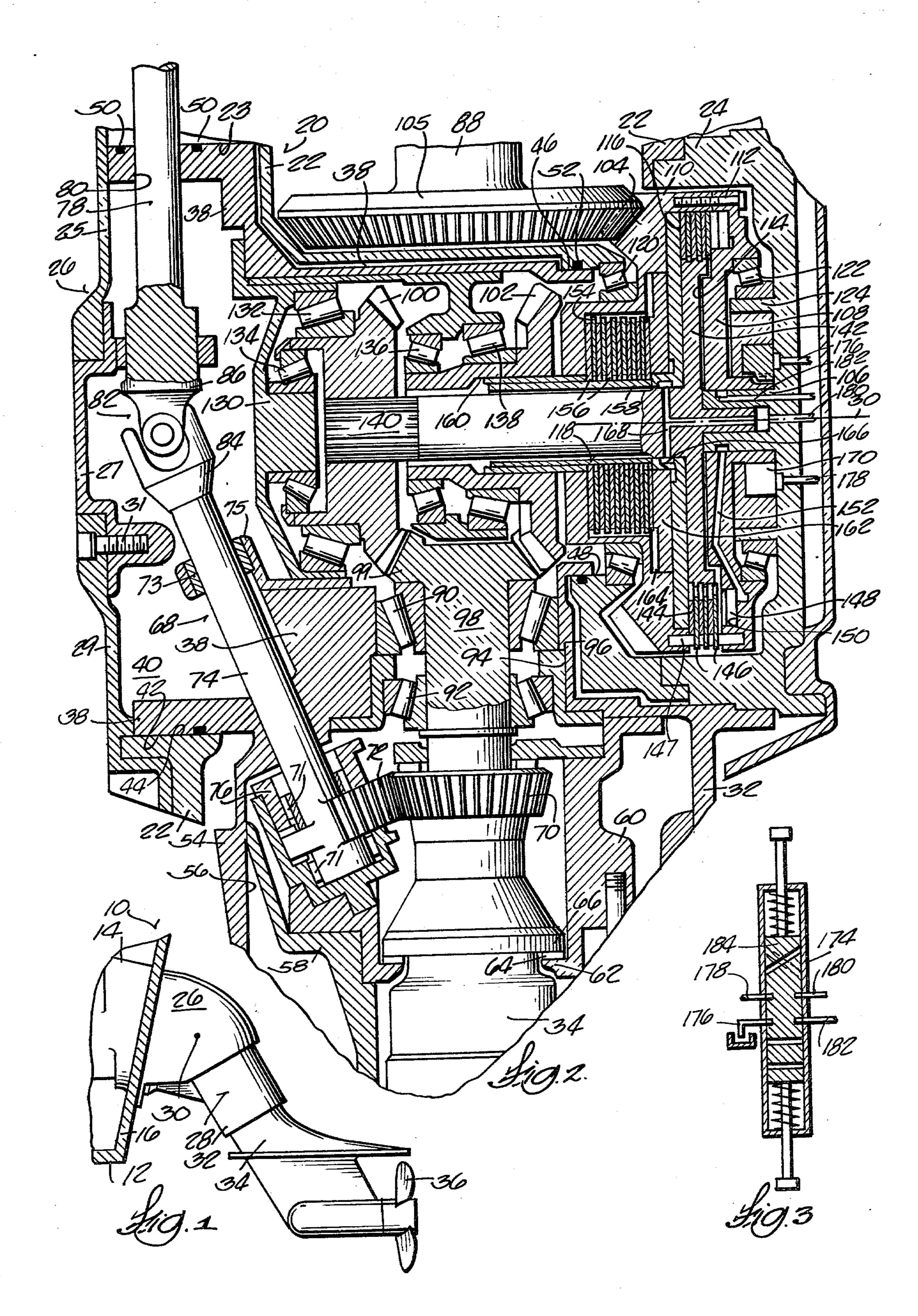
STERN DRIVE GEAR BOX AND CLUTCHING ARRANGEMENT
