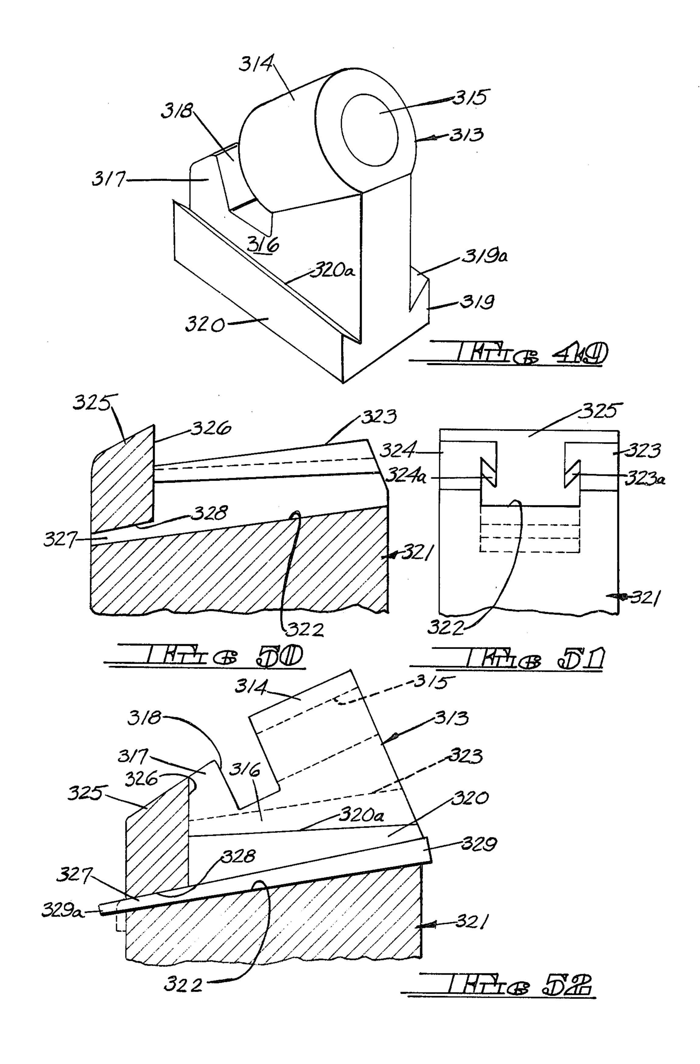
MEANS FOR REMOVABLY AFFIXING A CUTTER BIT MOUNTING LUG TO A BASE MEMBER ON THE DRIVEN ELEMENT OF A MINING MACHINE OR THE LIKE
