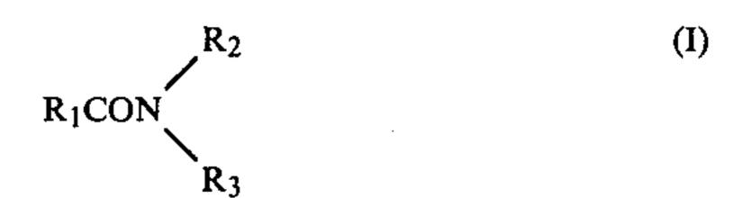
wherein R<sub>1</sub> represents an unsaturated hydrocarbon group having 18 to 23 carbon atoms, preferably 21 to 23 carbon atoms and at least one double bond and each of R<sub>2</sub> and R<sub>3</sub> represents a hydrogen atom or a lower alkyl group having 1 to 4 carbon atoms, preferably a hydrogen atom, a methyl group or an ethyl group.
