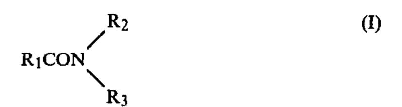
wherein R<sub>1</sub> represents a hydrocarbon group having 18 to 23 carbon atoms and at least one double bond and each of R<sub>2</sub> and R<sub>3</sub> represents a hydrogen atom or a lower alkyl group having 1 to 4 carbon atoms.
