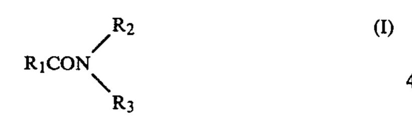
wherein R<sub>1</sub> represents a hydrocarbon group having 18 to 23 carbon atoms and at least one double bond and each of R<sub>2</sub> and R<sub>3</sub> represents a hydrogen atom or a 45 lower alkyl group having 1 to 4 carbon atoms.
