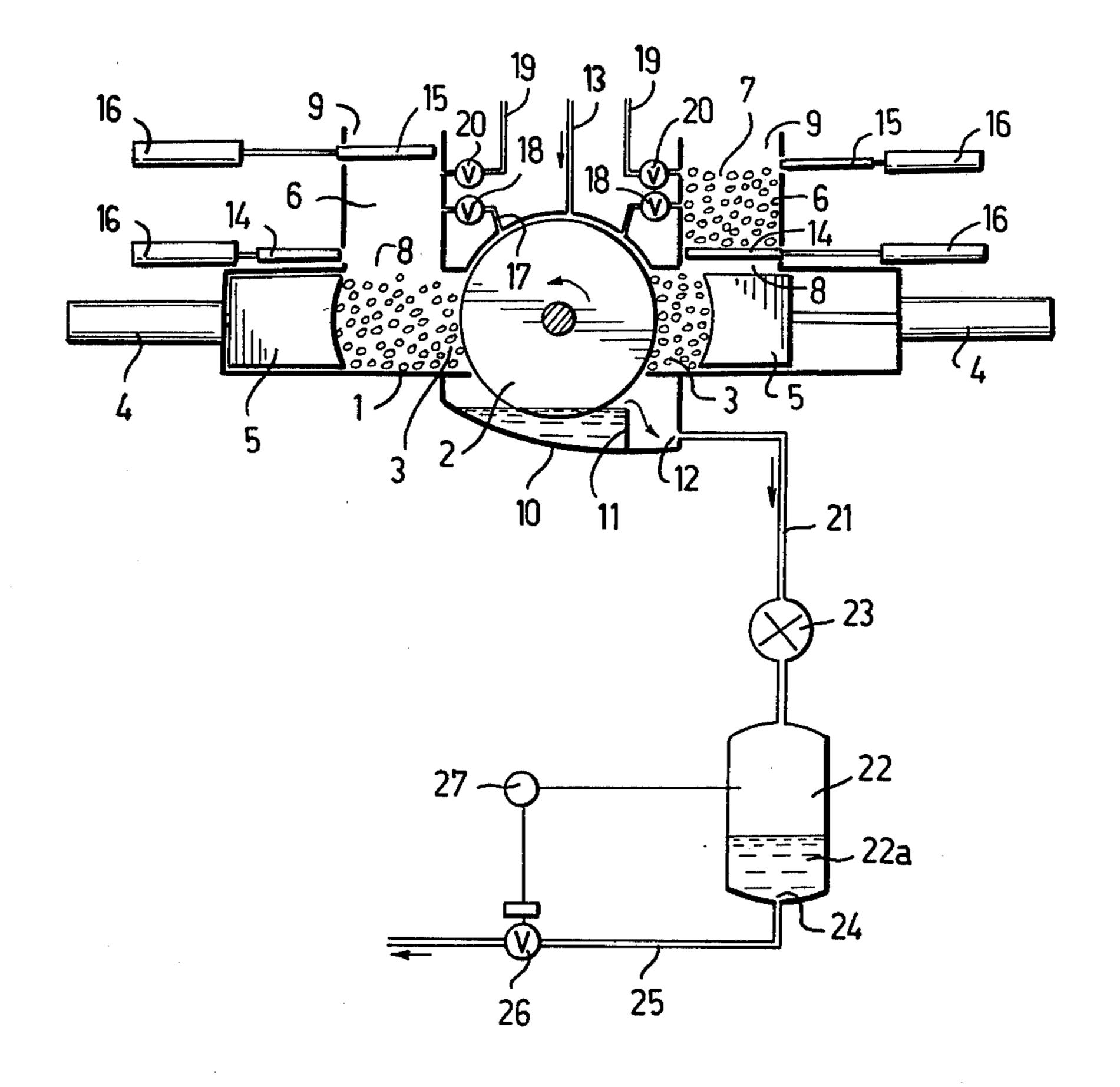
METHOD OF AND A GRINDER FOR GRINDING WOOD UNDER PRESSURE
