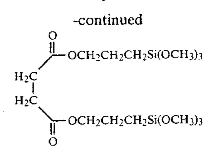
Accordingly, with the above background, it will now be desirable to describe a particular one-part RTV system in which the foregoing maleates, fumarates and succinates are superior self-bonding additives in the system. Such a system comprises 100 parts by weight of 15 the base silanol terminated diorganopolysiloxane polymer that was described previously and most preferably the polymer whose formula was given previously, that is, Formula 7.
