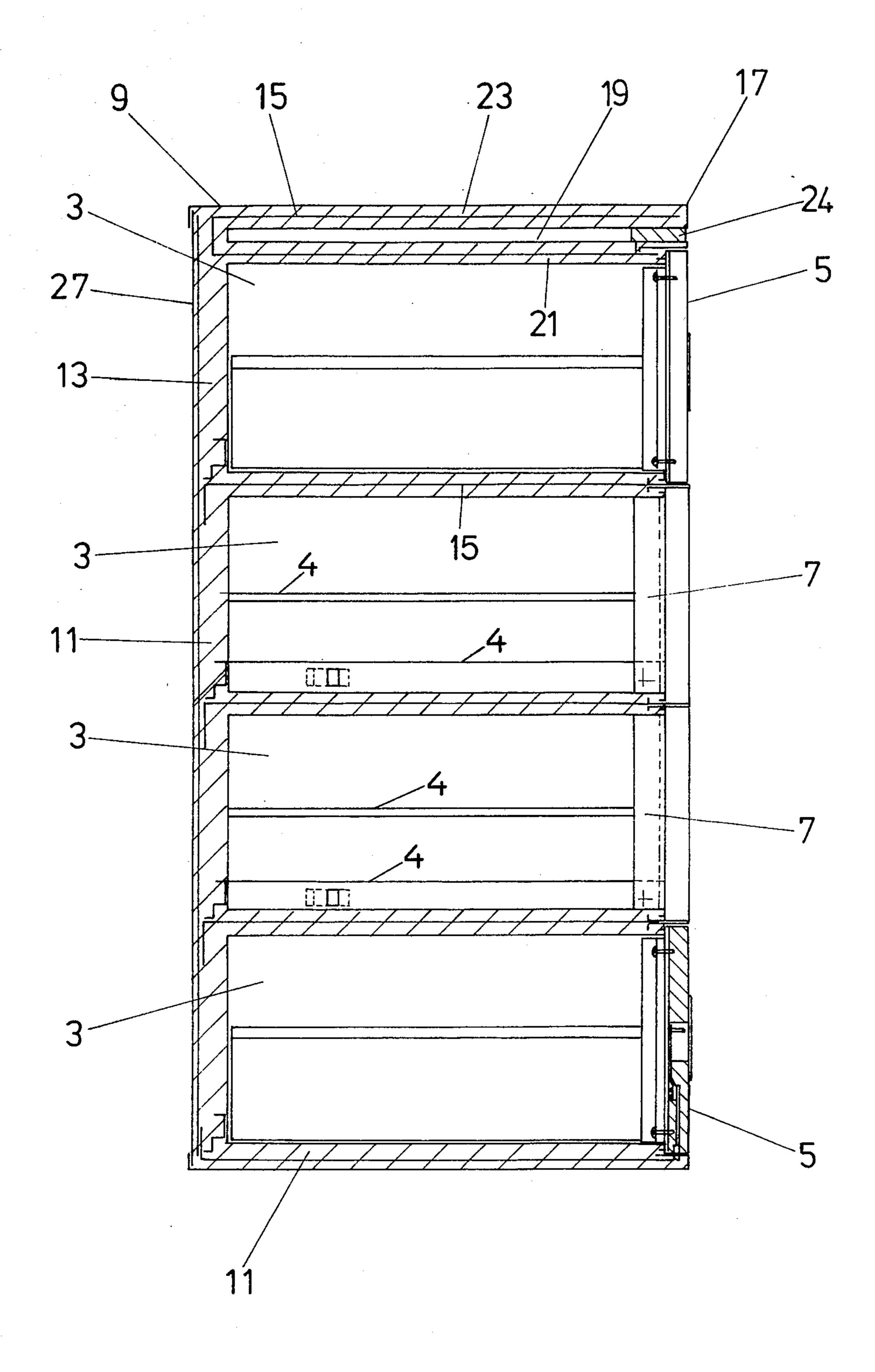
upper plate should break, the lower plate will provide heat protection.
