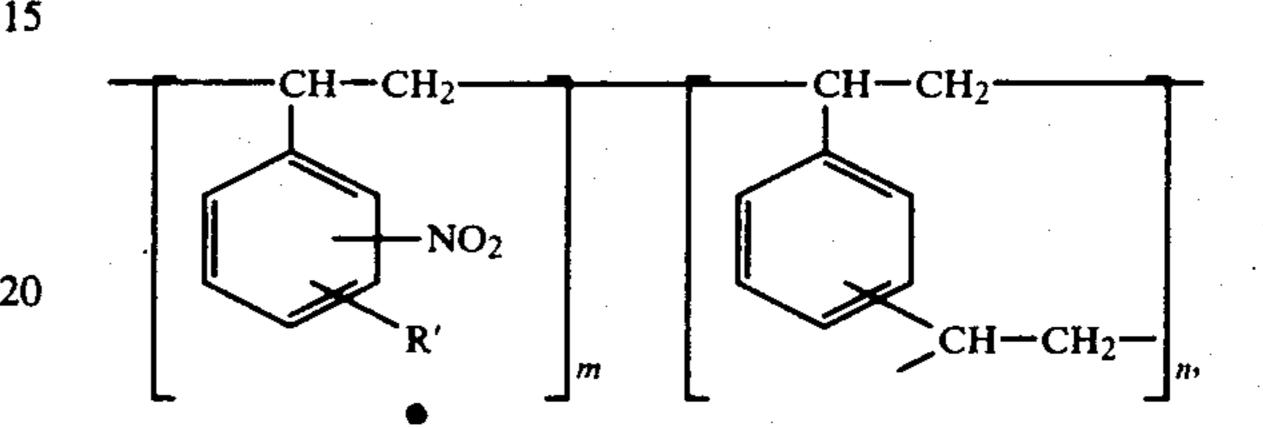
where R' is selected from the group consisting of H, NO<sub>2</sub>, COOH, SO<sub>3</sub>H, P(O)(OH)<sub>2</sub>, P(O)H(OH), m is from 60 to 99, and n is from 40 to 1, consisting in that the cross-linked polymers having the general formula
