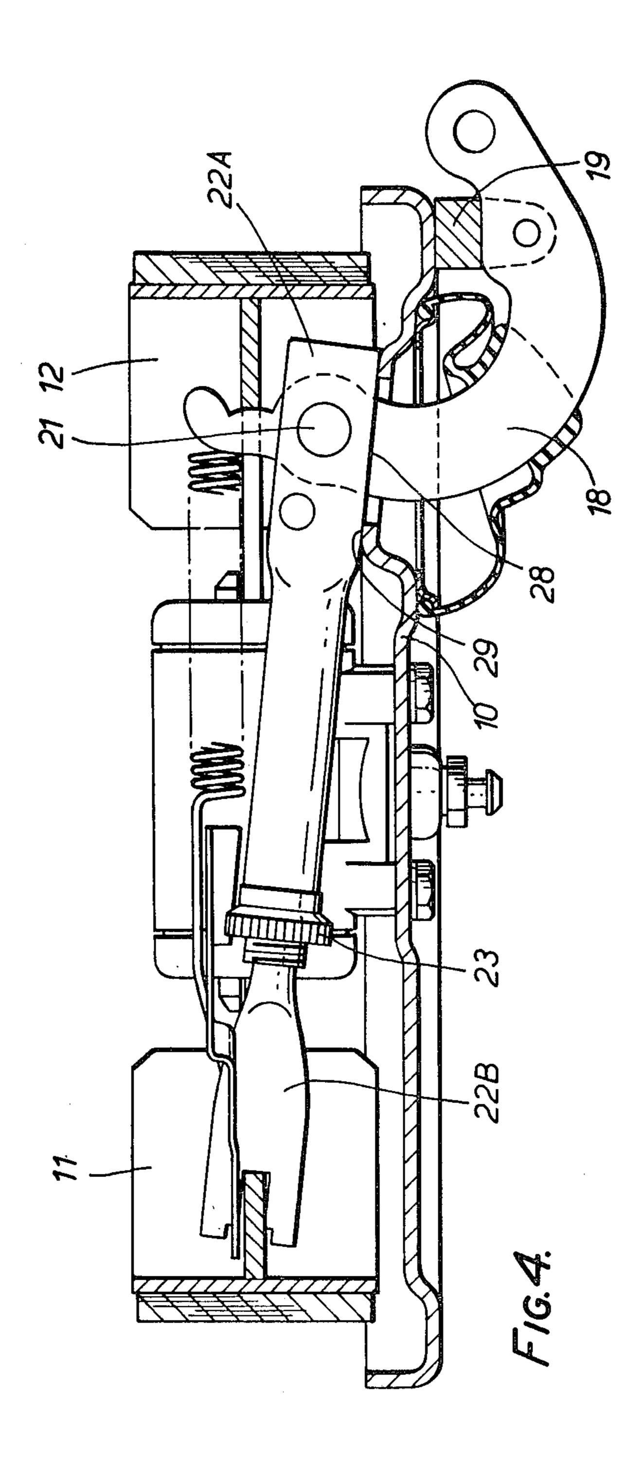
rotation of the auxiliary actuator lever, the strut slides along said surface portion. The surface portion is preferably formed by pressing the back plate.
