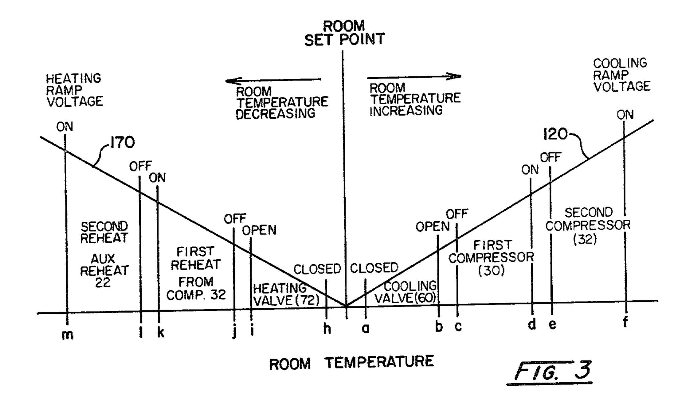
CONTROL SYSTEM FOR AN AIR CONDITIONING SYSTEM HAVING SUPPLEMENTARY, AMBIENT DERIVED COOLING
