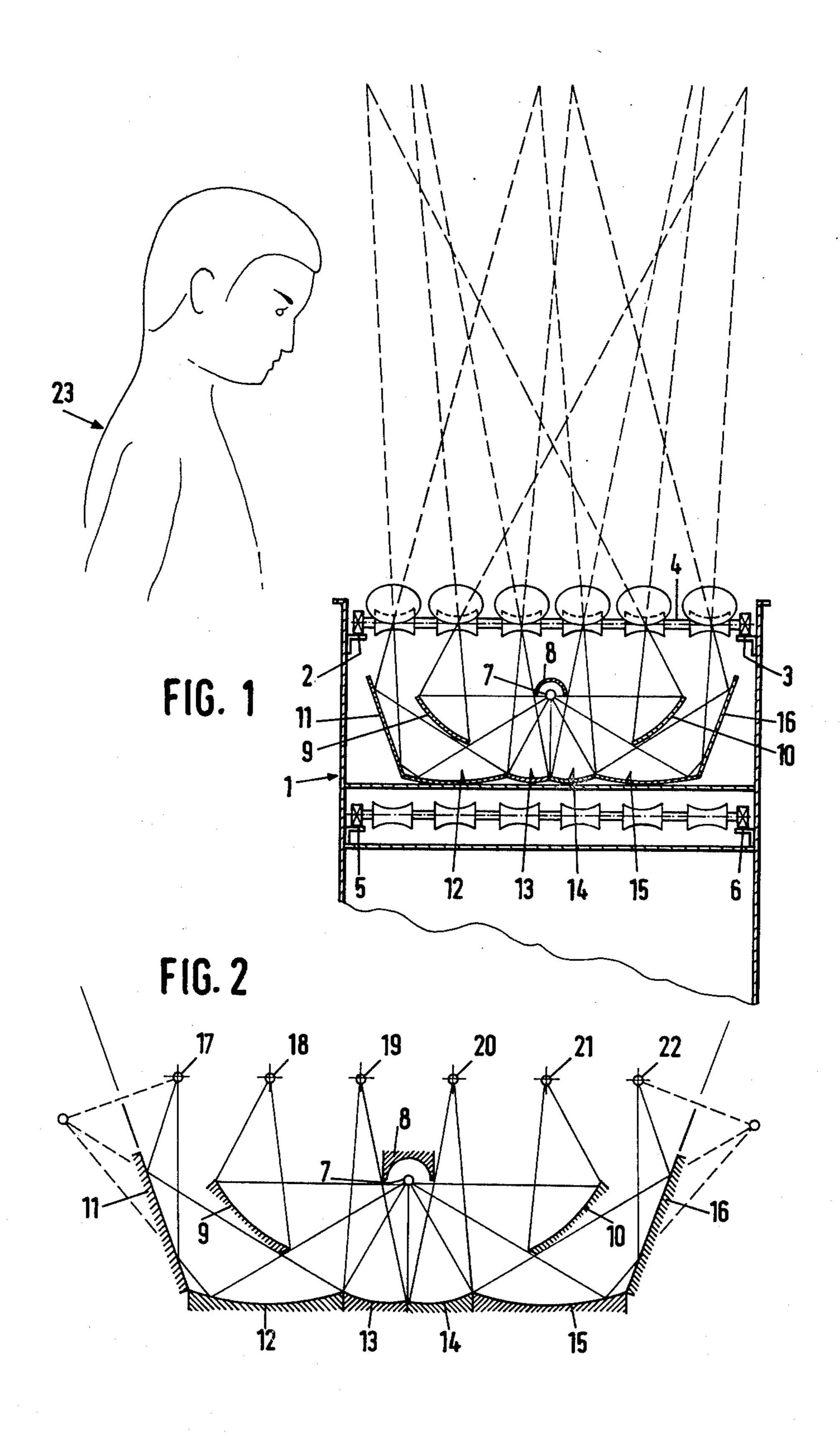
FIG. 2 shows, diagrammatically, the lighting system used in the device of FIG. 1.
