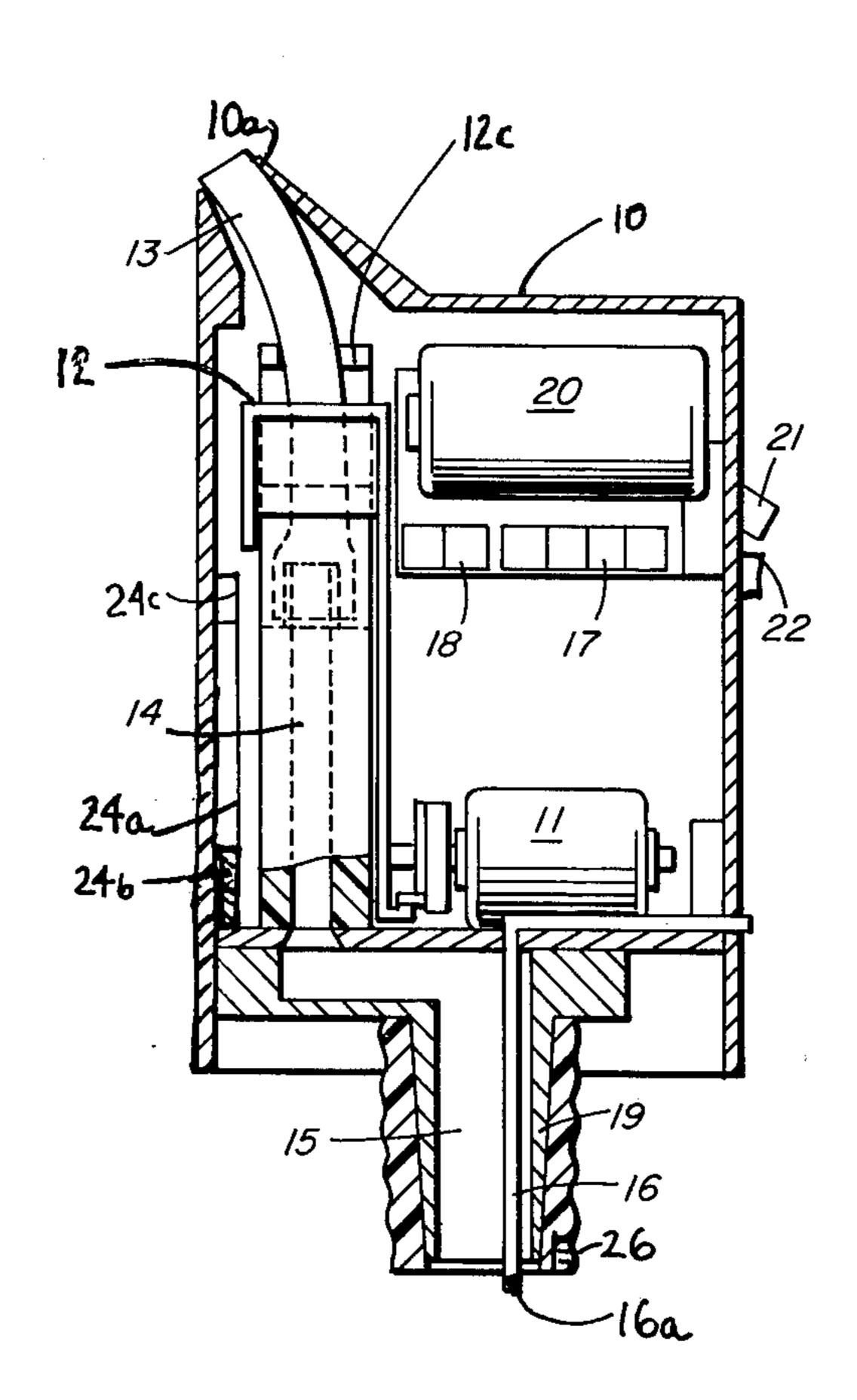
U.S. Patent 4,265,370 May 5, 1981 Sheet 1 of 2 ,12c F/G. / F1G. 2 \_120 13-12b 0 BOTTLE SHOT **TIPPING** 18 COUNT COUNT **SWITCH** DISPLAY DISPLAY FIG. 3 24 0193 POUR VALVE 100 ON/OFF .MOTOR LOGIC CIRCUIT SWITCH 23 DC SOURCE MAGNETIC FIG. 4 POUR REED 20 **ADJUST SWITCH**
