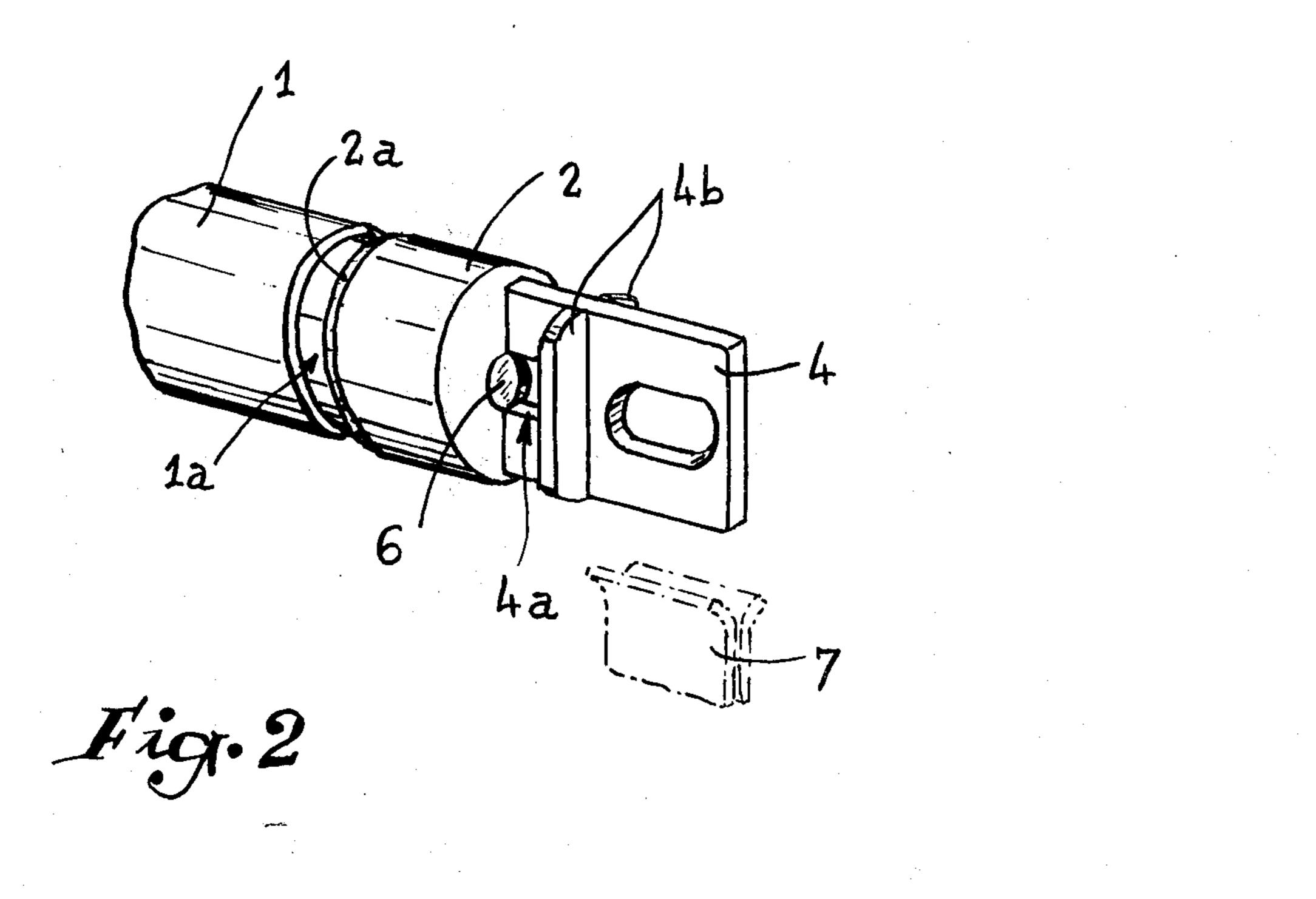
The present invention relates to fuse cartridges of the kind comprising a tubular insulating body having a 5 metallic head at each end, these heads being electrically connected with each other by means of fusible wires or elements disposed within the insulating body. The latter is generally filled with an appropriate arc-quenching substance, such as silica sand, in which the fusible ele- 10 ments are embedded.
