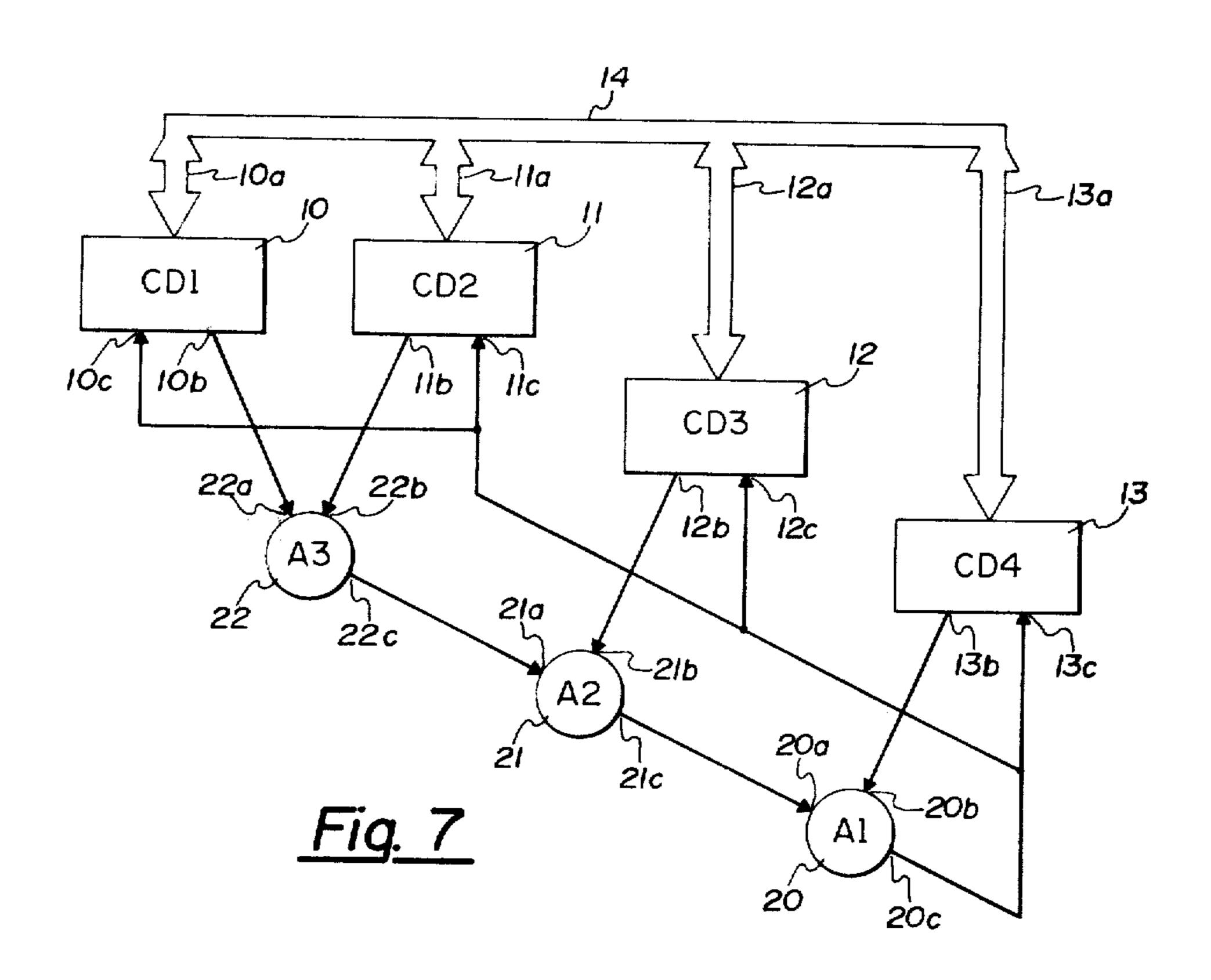
DATA PROCESSING SYSTEM INCORPORATING ARBITERS AND SELECTORS TO ALLOCATE TRANSMISSIONS BY MULTIPLE DEVICES ON A BUS
