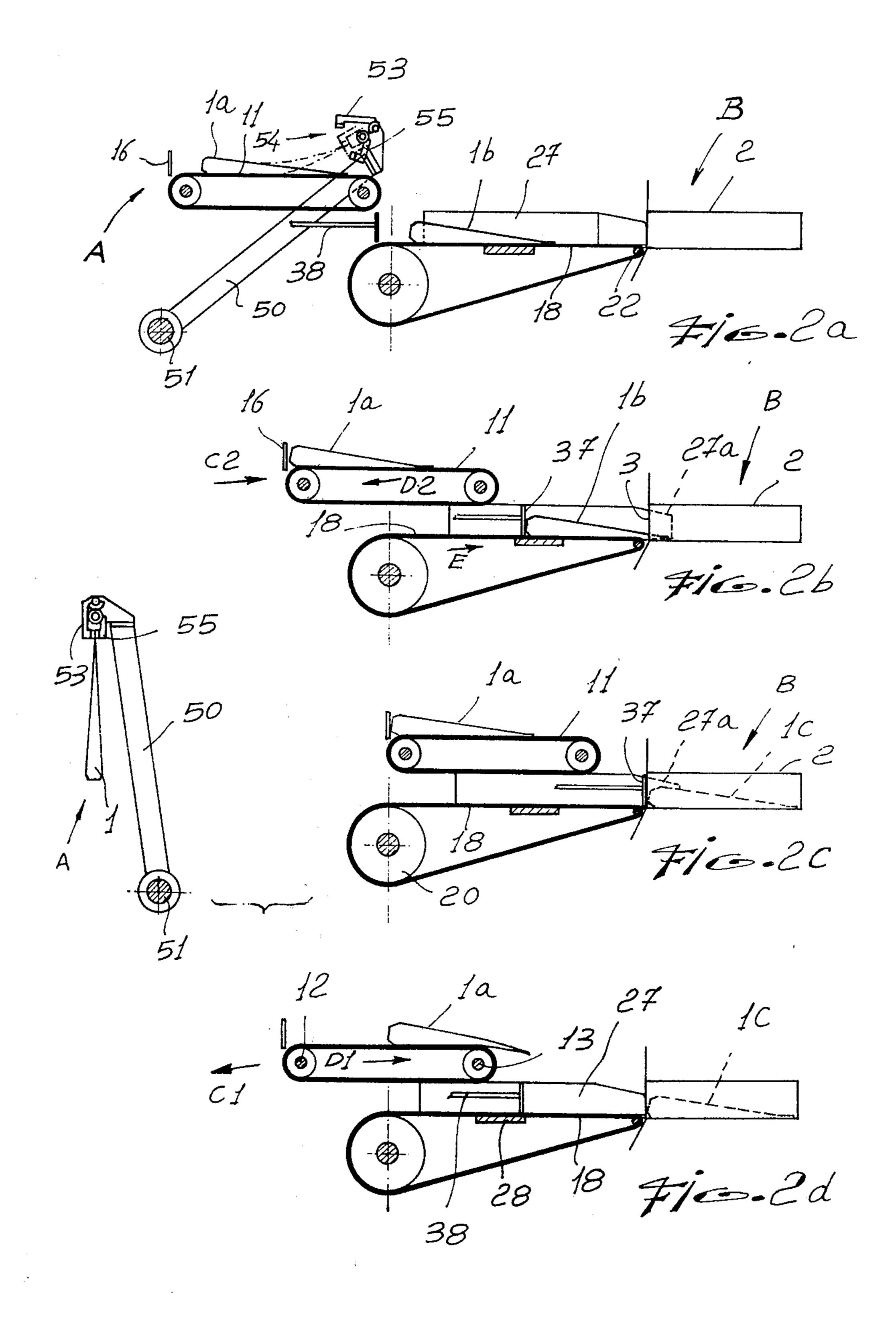
inserting a bag deposited thereon into one of said boxes positioned at said second station.
