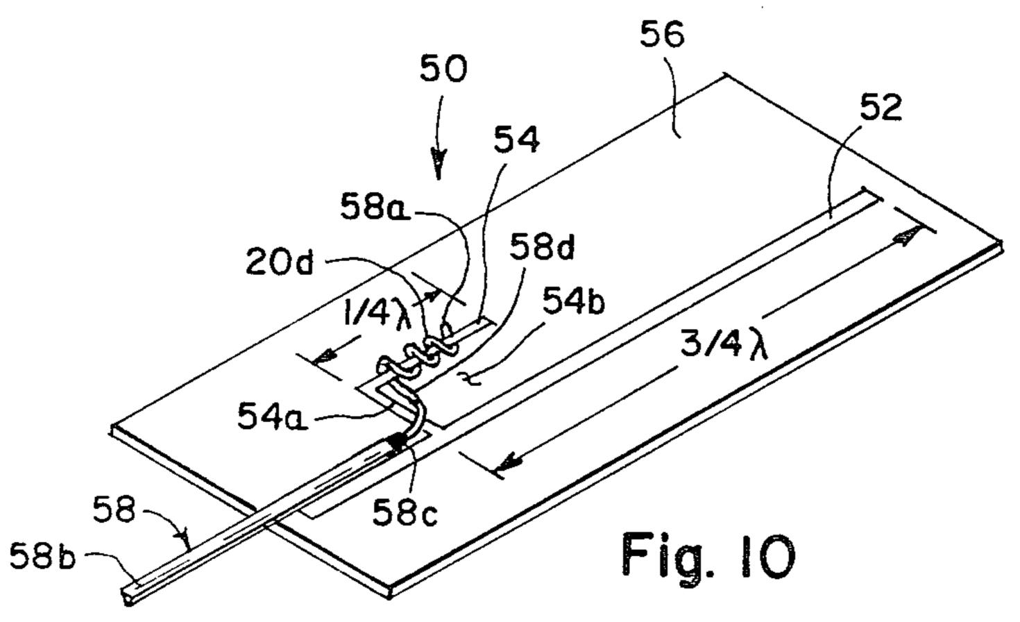
This invention relates to an antenna and, more particularly, to a broadbanded antenna of the J-configuration having a unique method of feed.
