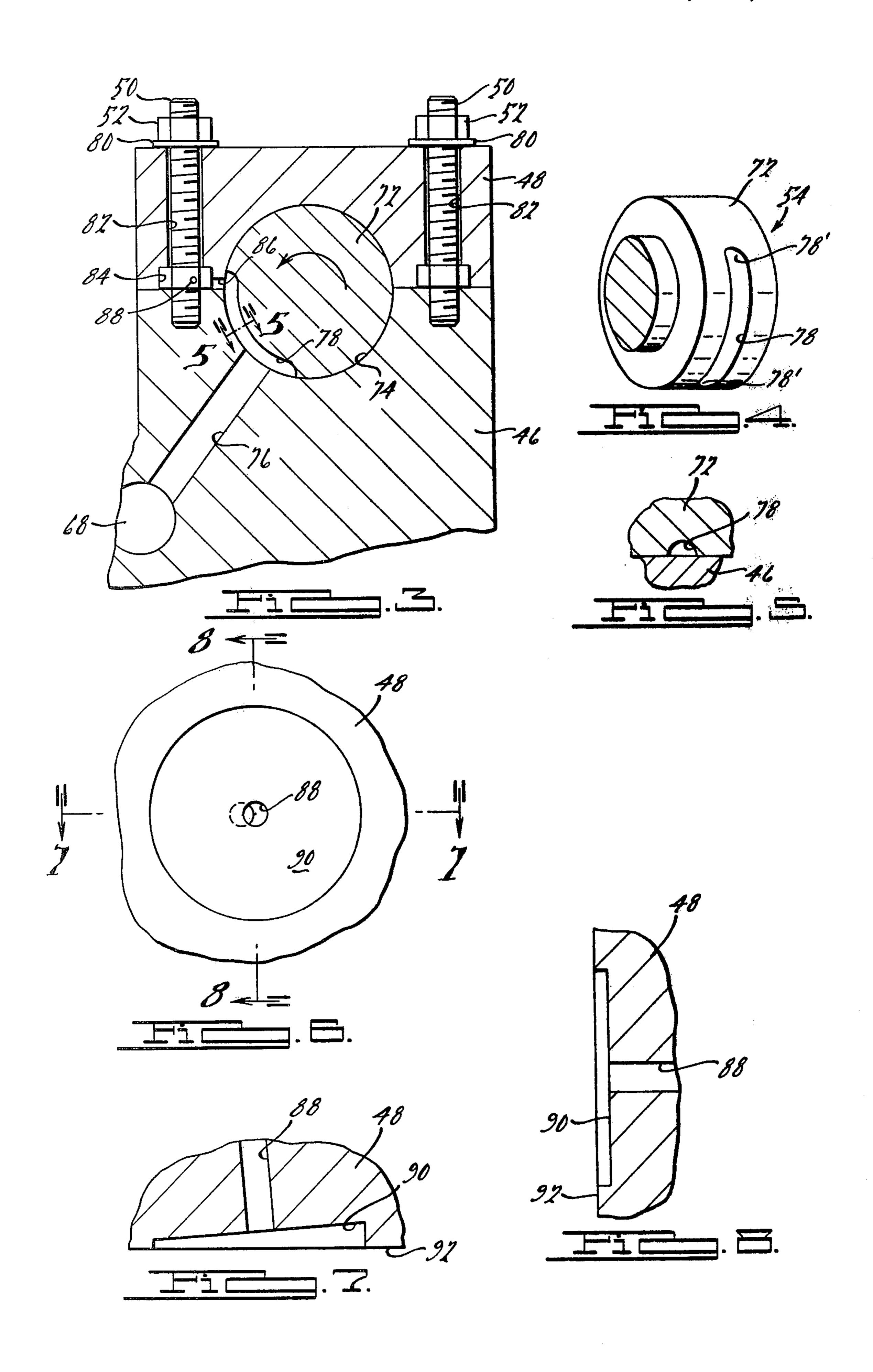
This application relates to an improved lubricating apparatus for cam lobes and particularly to such a sys- 5 tem to supply pressurized oil intermittently to a small orifice opening with its axis directed toward the cam lobe.
