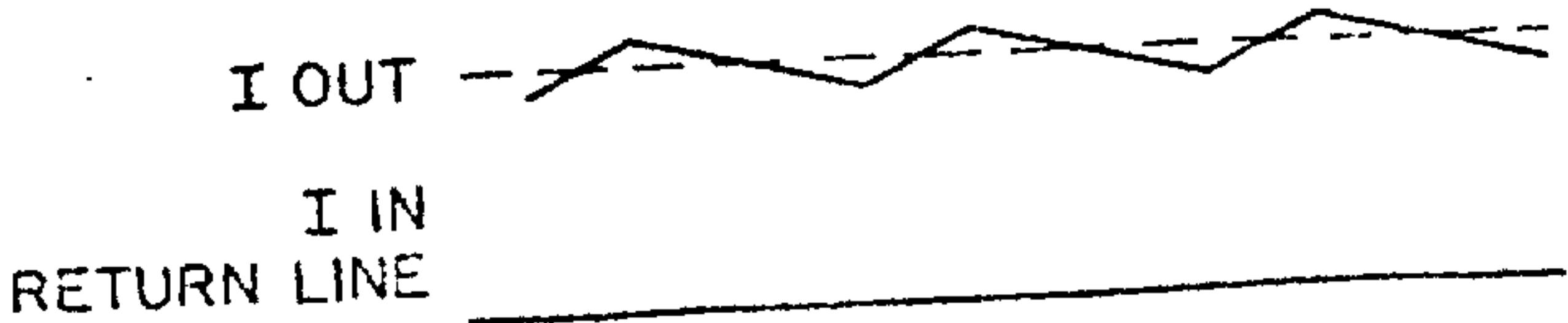
FIG. 3H E_{IN} RETURN CURRENT WITH FLYBACK CONTROL
