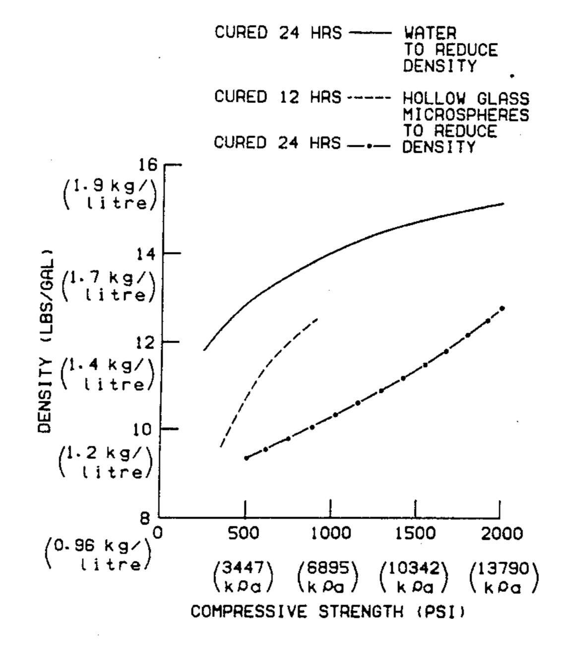
API CLASS A CEMENT 1000 FT (305m) API RP 10B SIMULATED WELL
