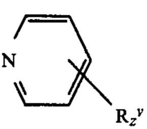
in which  $R^{\nu}$  is hydrogen or a hydrocarbyl radical having from 1 to 3 carbon atoms and z has a value from 0 to 4.
