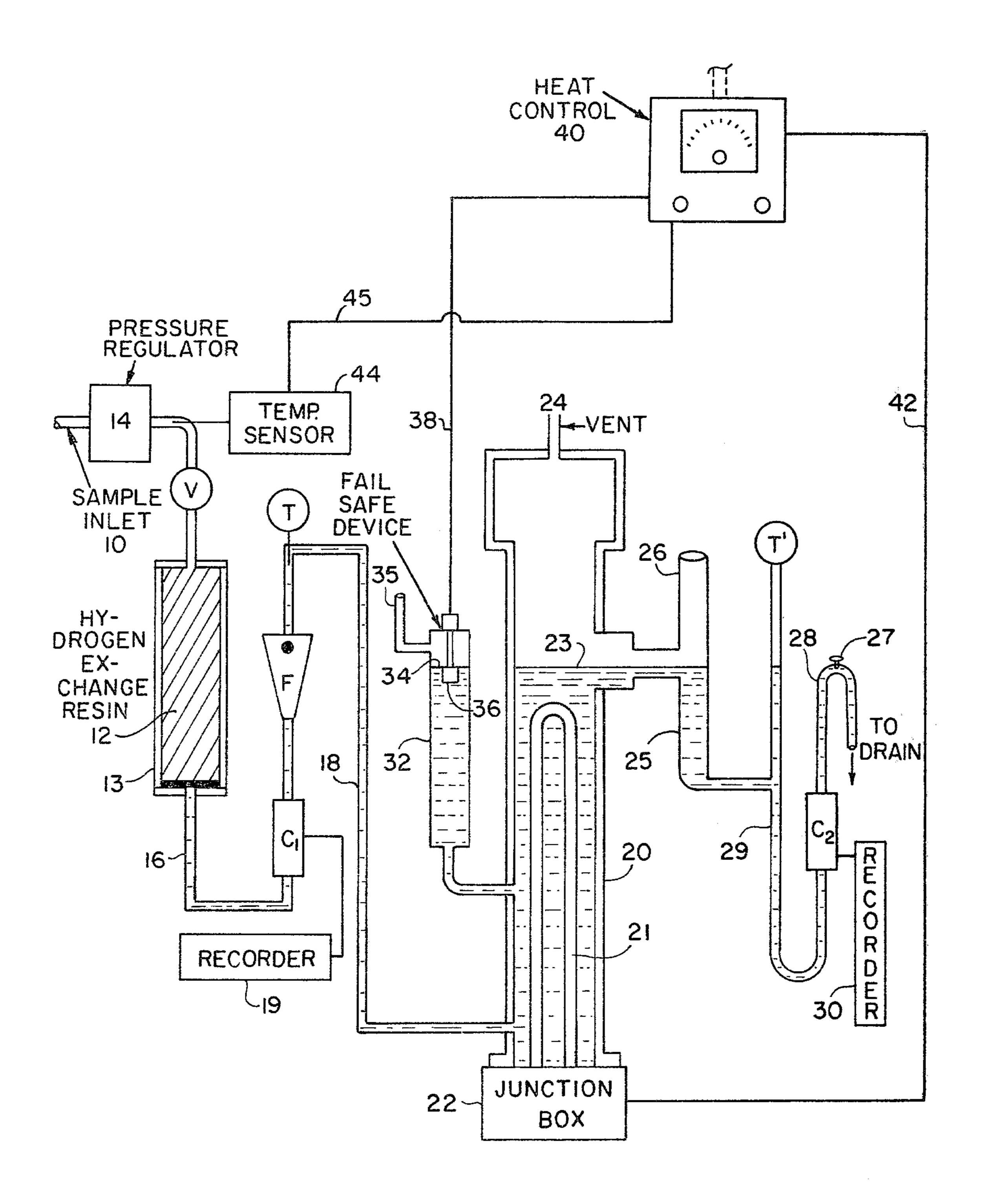
APPARATUS FOR AND METHOD OF DETERMINING CONTAMINANTS ON LOW PRESSURE CONDENSATE
