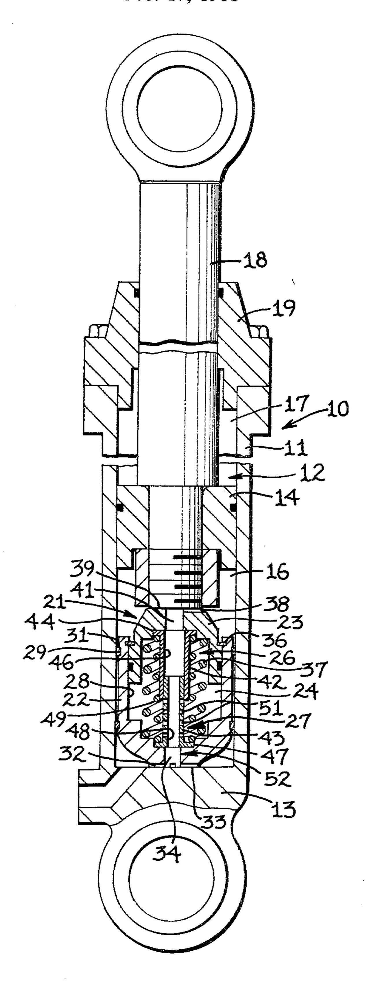
slidably extending through an end cap 19 and having an end connected to the piston.
