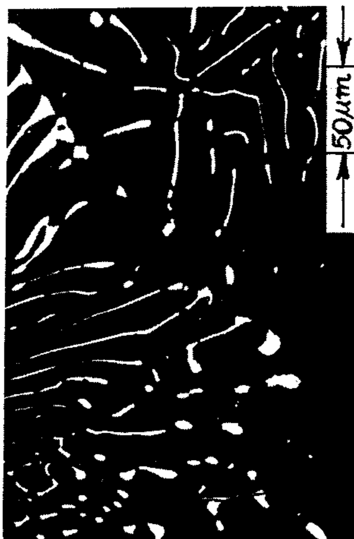
MC TYPE CARBIDES IN STEEL C11V
