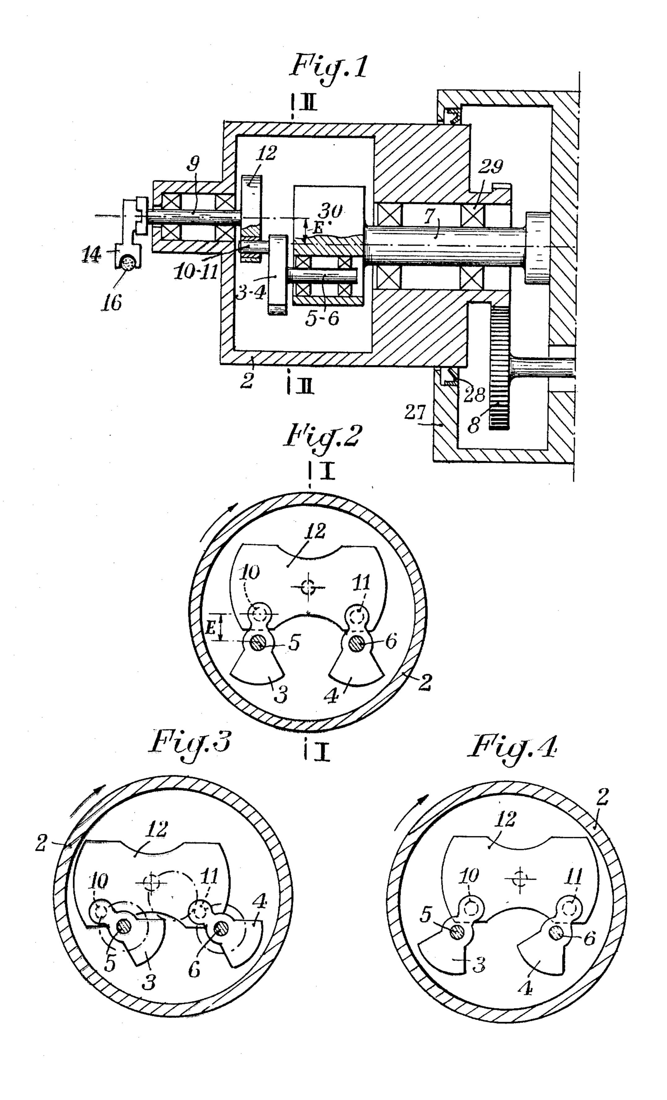
annular seal 28. For this purpose, a bearing 29 provided in the rear portion of case 2 permits the mounting of the latter on the shaft 7.
