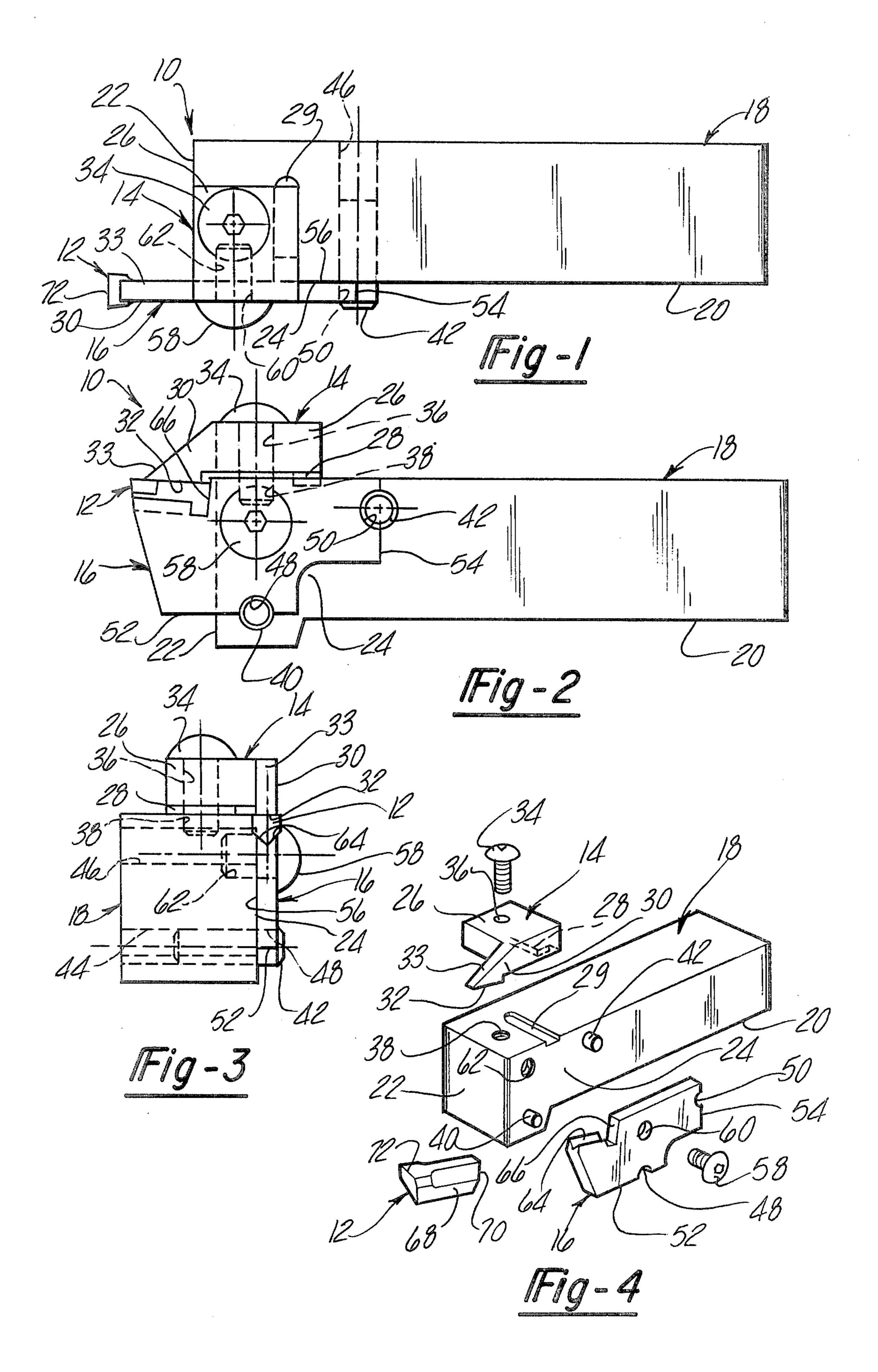
edge 72 of the insert 12 constitutes the widest portion of the insert which may be formed of tungsten carbide or a similar hard cutting material.
