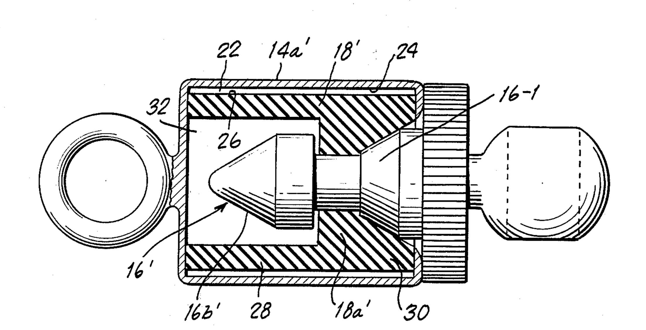
FIG. 3 is an exploded view of the parts of the clasp of FIG. 2.
