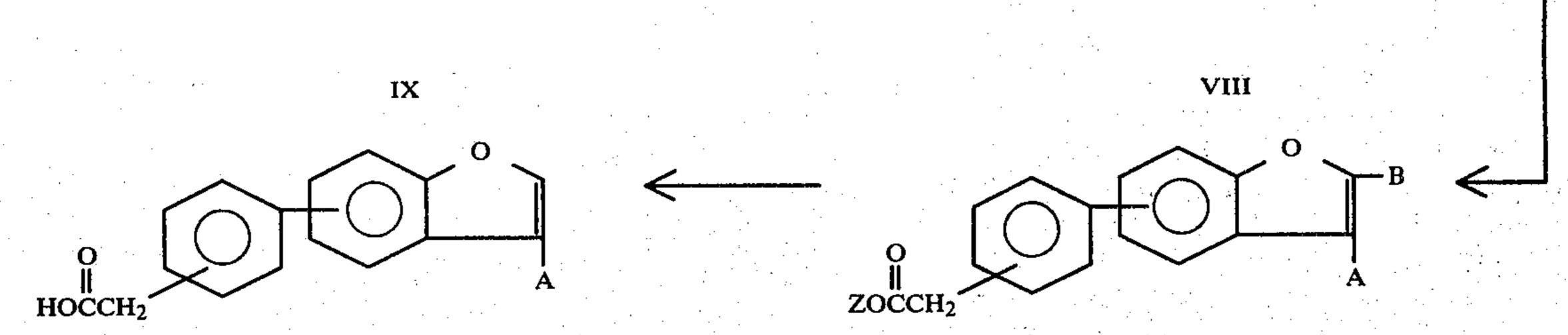
wherein Z is hydrogen or alkyl of one to four carbon atoms, A is methyl or ethyl and B is hydrogen or ethyl carboxylate. The intermediate compounds VII, VIII 15 and IX are novel and form separate aspects of the present invention. The reaction to form the compounds VII is generally run at reflux, in an inert solvent in the presence of a base such as sodium carbonate or, when ethyl  $\alpha$ -chloroacetoacetate is used, the preferred base is so-20 dium ethoxide.
