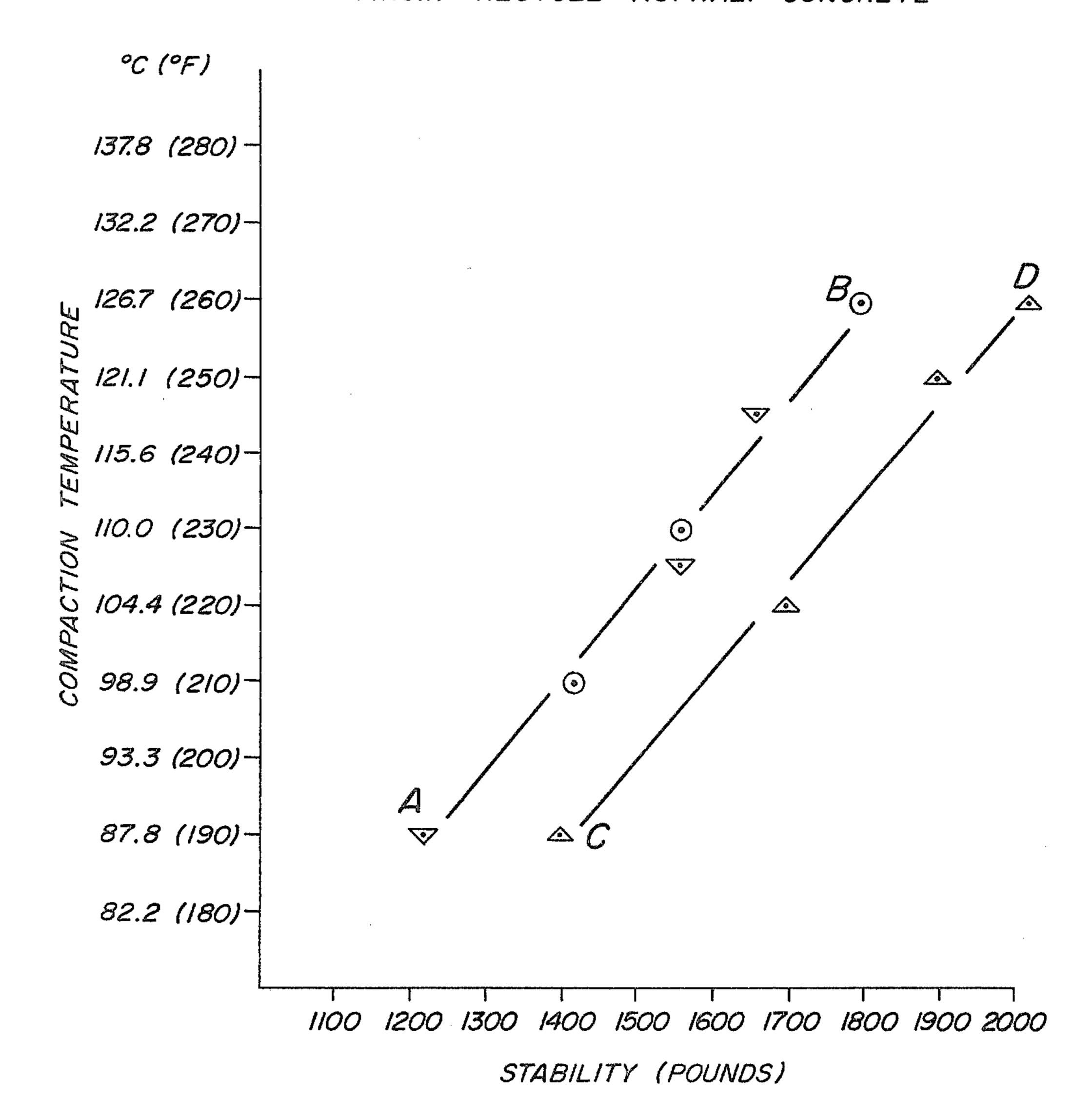
100% VIRGIN ASPHALT CONCRETE MIXTURE OF EXAMPLE I
