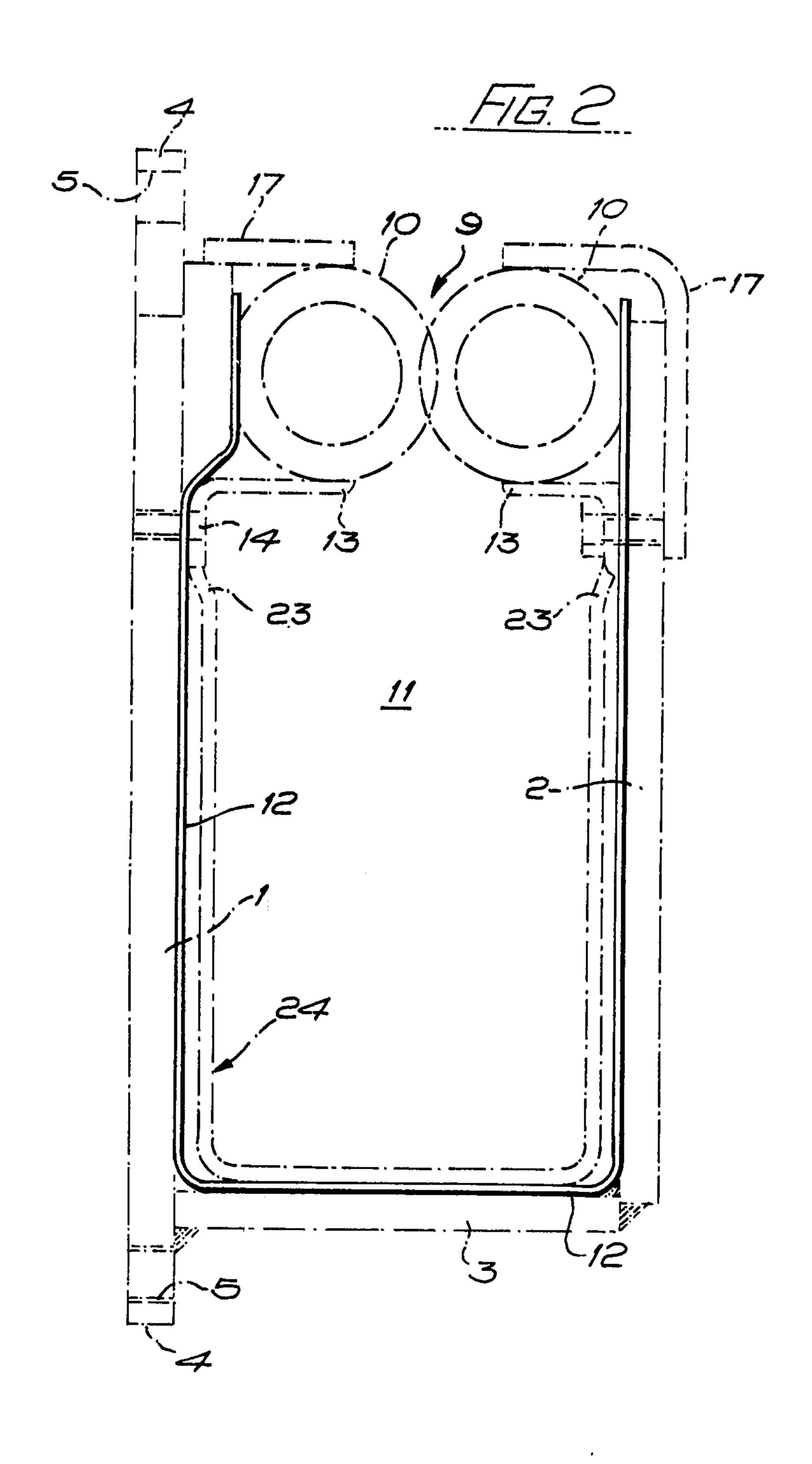
This invention relates to a conduit length to be joined in use to adjacent ends of similar conduit lengths to 5 form an electrical power supply conduit when housing one or more electrical conductors, for the supply of electrical energy to electrical machines adjacent the conduit.
