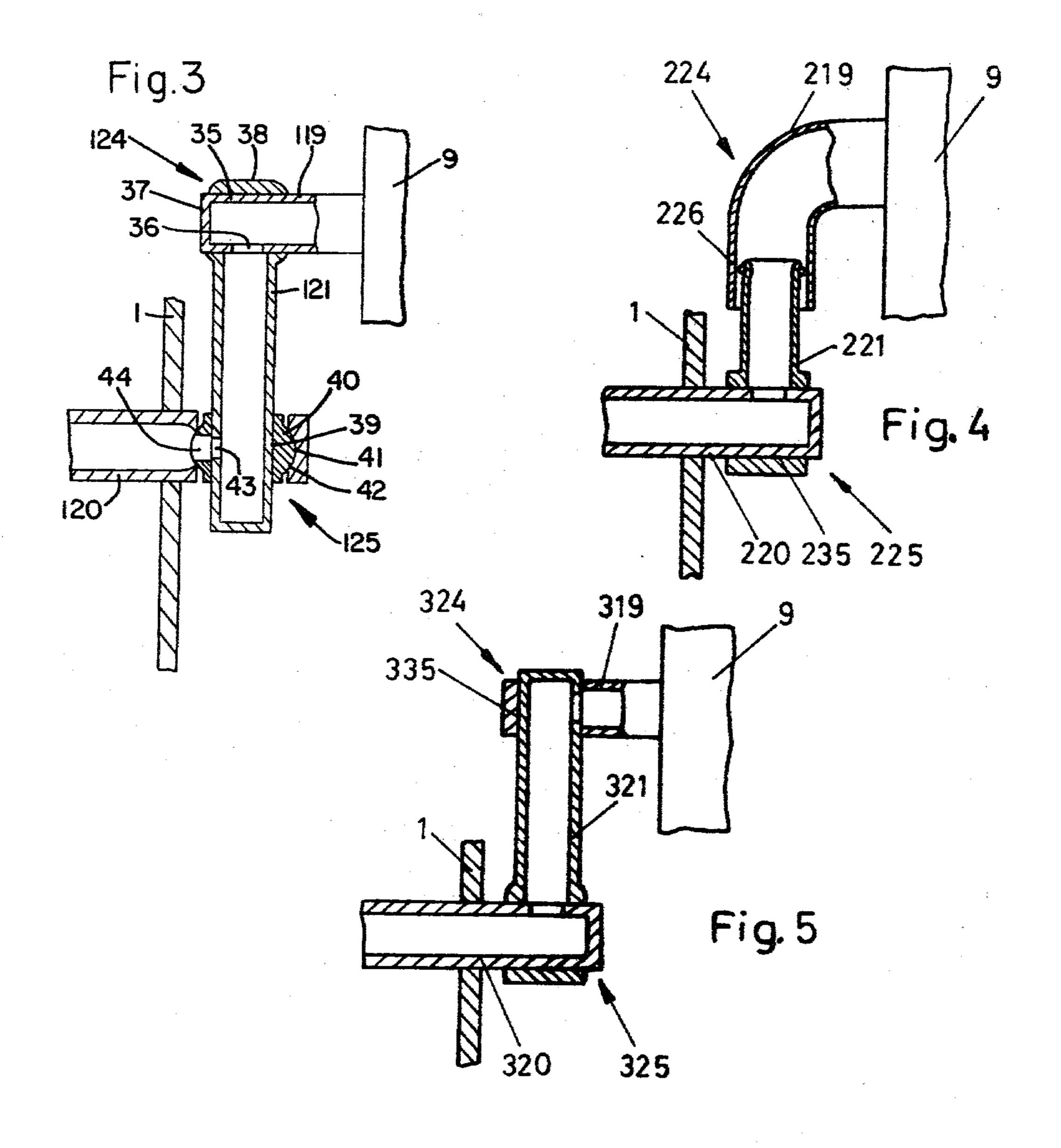
joint has at least one rotary axis which coincides with the axis of the connecting pipe and the other joint has at least one rotary axis coinciding with one pipe connector
