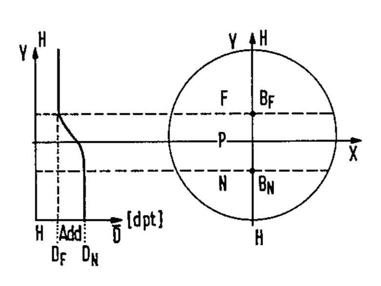
H Main meridian = Umbilical point line or quasi - umbilical point line Far-sight field Progression zone Near - sight field Optical far reference point = Site for the prescribed far correction BN Optical near reference point = Site for the prescribed near correction Surface refraction value in the far-sight field DN Surface refraction value in the near-sight region Average surface refraction value Add Near addition =  $D_N - D_F$
