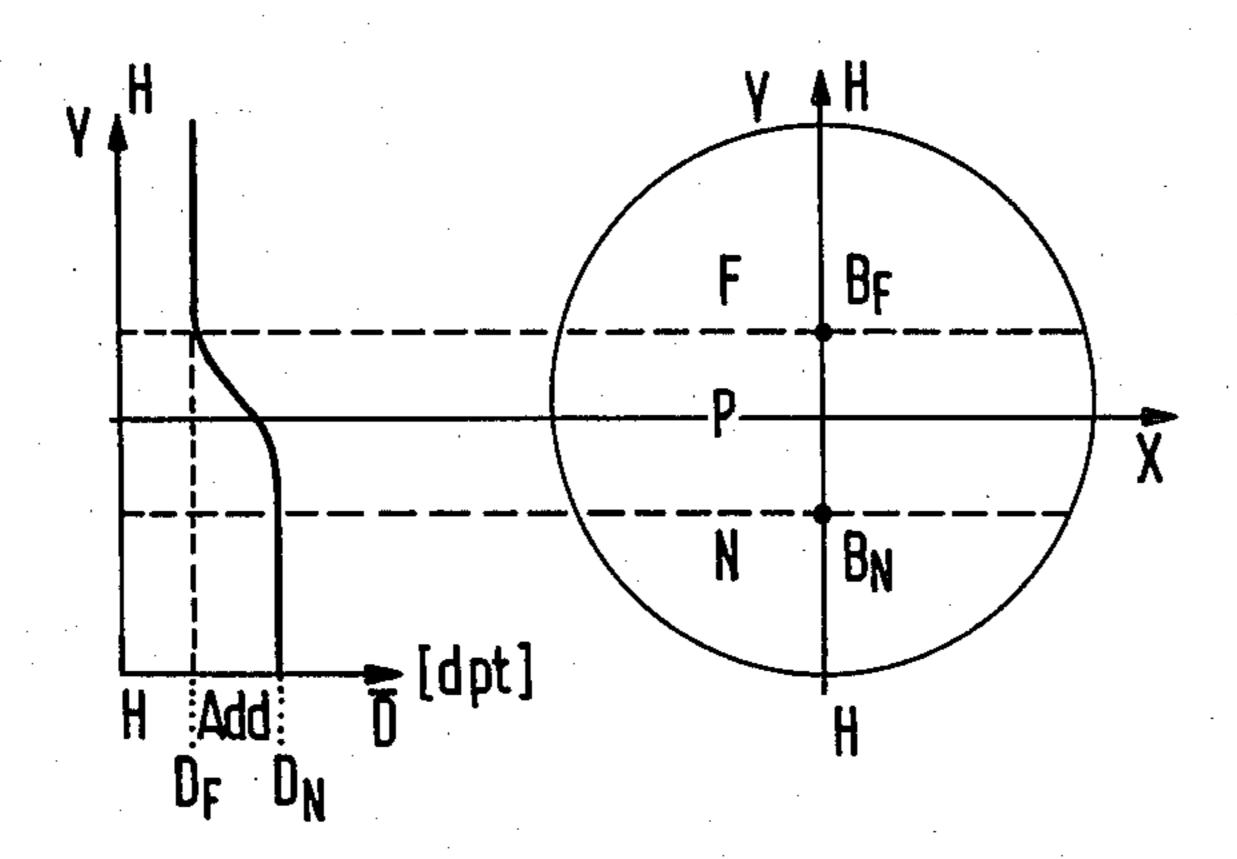
Main meridian = Umbilical point line or quasi - umbilical point line Far-sight field Progression zone Near - sight field BF Optical far reference point = Site for the prescribed far correction BN Optical near reference point = Site for the prescribed near correction DF Surface refraction value in the far-sight field DN Surface refraction value in the near-sight region Average surface refraction value Add Near addition =  $D_N - D_F$
