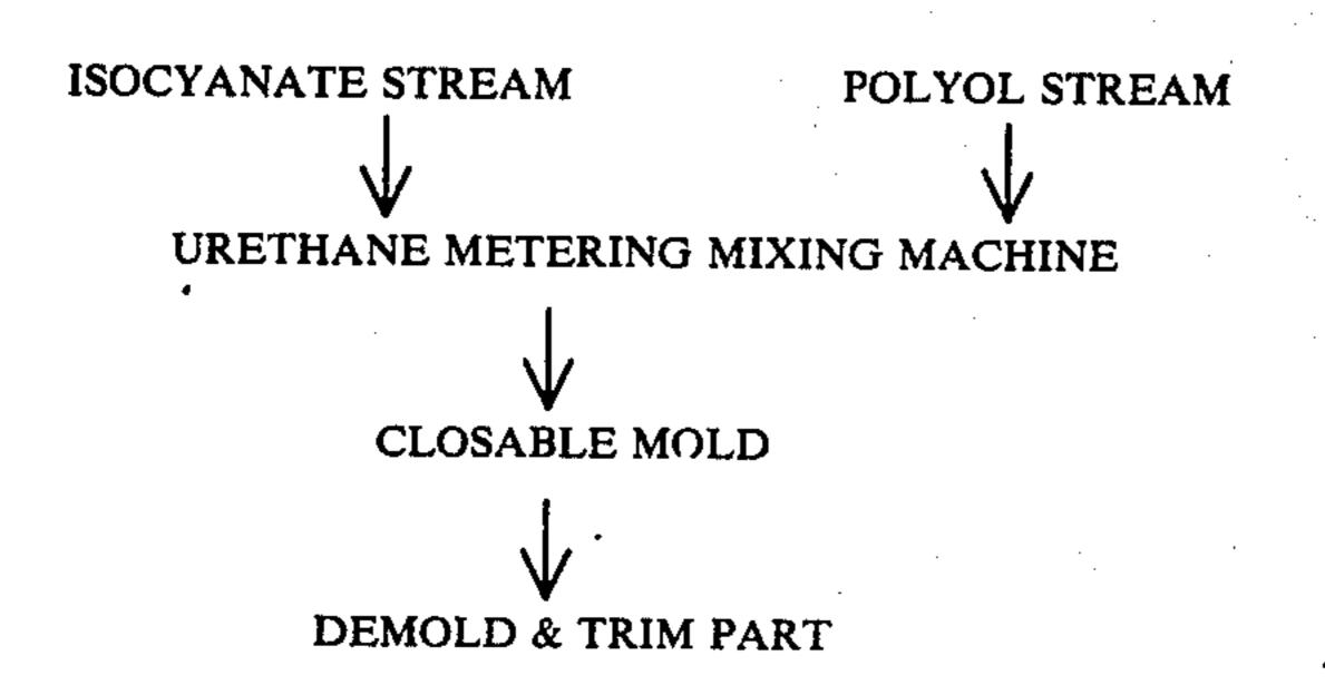
The microcellular and solid elastomers produced in accordance with the present invention are useful in the production of automotive exterior body panels, tractor and snowmobile bodies, and the like.
